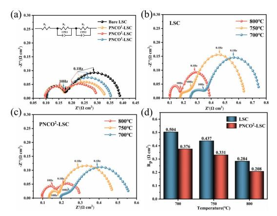
Fig. 4 (a) Equivalent circuit diagrams, and Nyquist plots of single cells with different infiltration loads at 800 °C, (b) Nyquist plots of LSC, (c) Nyquist plots of PNCO<sup>2</sup>–LSC, (d) polarization resistance of bare LSC and PNCO<sup>2</sup>–LSC at different temperature.
