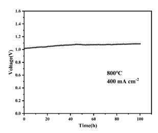
Fig. 5 Long-term stability of PNCO<sup>2</sup>-LSC composite oxygen electrode cells.
