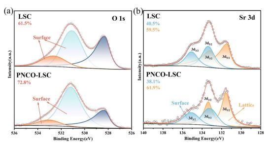
Fig. 6 XPS spectra of (a) O 1s, (b) Sr 3d for LSC and PNCO<sup>2</sup>-LSC.
