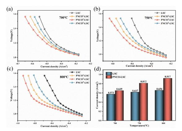
Fig. 3 J-V curves of (a) 700 °C, (b) 750 °C, (c) 800 °C, (d) current density of bare LSC and PNCO<sup>2</sup>-LSC at different temperatures.
