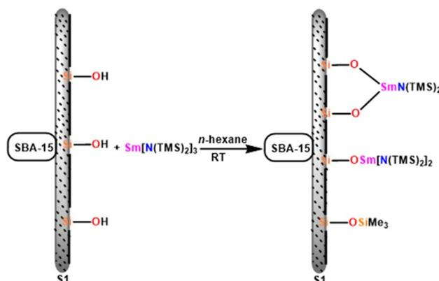
Scheme 35 Immobilization of Sm[N(SiMe<sub>3</sub>)<sub>2</sub>]<sub>3</sub> onto mesoporous SBA-15.
