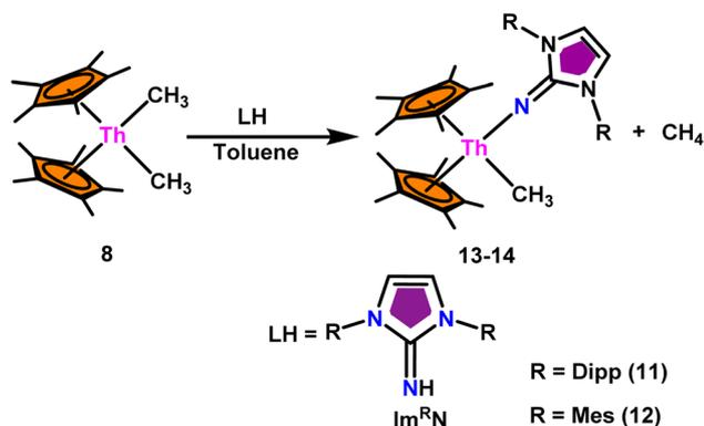
**Scheme 11** Synthesis of  $\text{Cp}^*_2\text{Th}(\text{L})(\text{Me})$  (**13–14**).
