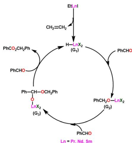
Scheme 20 The plausible mechanism of **33** catalyzed Tishchenko reaction.
