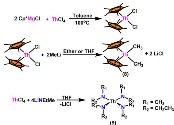
Scheme 6 Synthesis of  $\text{Cp}^*\text{ThMe}_2$  (8) and  $\text{Th}(\text{NEtMe})_4$  (9).
