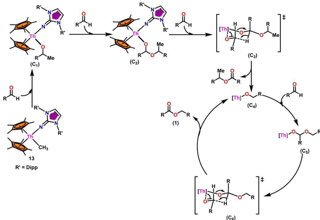
Scheme 12 Tishchenko reaction mediated by complex  $\text{Cp}^*_2\text{Th}(\text{Im}^{\text{Dipp}})(\text{Me})$  (13).
