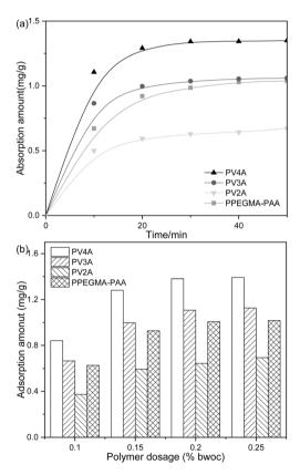
Fig. 9 The adsorption performance of PV4A, PV3A, PV2A and PPEGMA-PAA onto cement. (a) Adsorption amount over time at 0.15% bwoc dosage; (b) adsorption saturation amount against polymer dosage.
