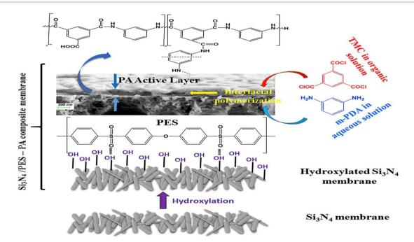
Fig. 9 TFC synthesis based on  $Si_3N_4$ /polyethersulfone (PES) composite membrane. Reprinted with the permission of ref. 118, copyright 2024, Elsevier.
