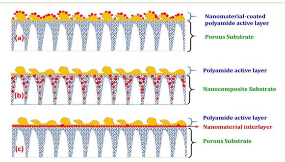
Fig. 3 Schematic illustrations demonstrating typical structures of nanomaterial-modified PA TFC membranes: (a) TFC membrane with nanomaterial-coated PA surface layer, (b) TFC membrane with nanocomposite substrate and (c) TFC membrane with nanomaterial interlayer. Reprinted with the permission of ref. 32, copyright 2024, 2024 Elsevier.
