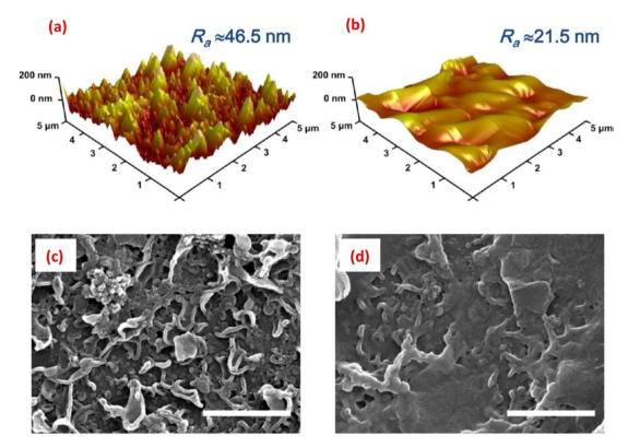
Fig. 14 AFM height images of (a) the pristine, uncoated polyamide (PA) and (b) the  $GO_{10}$ -coated PA membranes; and the SEM images of (c) the pristine PA and (d) the  $GO_{10}$ -coated PA membranes, (scale bar  $= 1 \mu m$ ). Reprinted with the permission of ref. 29, copyright 2024, American Chemical Society.
