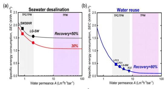
Fig. 15 Relationship between specific energy consumption (SEC, kW h m<sup>-3</sup>) and product flow in the context of (a) seawater desalination and (b) water reuse. Reprinted with the permission of ref. 29, copyright 2024, American Chemical Society.
