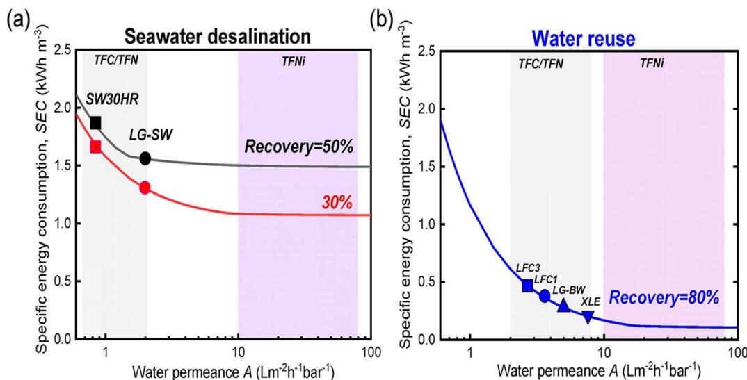
Fig. 15 Relationship between specific energy consumption (SEC,  $\text{kWh m}^{-3}$ ) and product flow in the context of (a) seawater desalination and (b) water reuse. Reprinted with the permission of ref. 29, copyright 2024, American Chemical Society.
