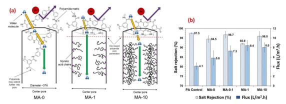
Fig. 8 (a) Schematics of water transport through the pores of zirconium-based porphyrinic MOFs (PCN-222 nanorods) with increasing modifier loading (myristic acid, MA, at 0, 0.1, 1 and 10%), and (b) salt rejection and water flux results for MA-modified and pristine membrane reprinted with the permission of ref. 89, copyright 2024, American Chemical Society.
