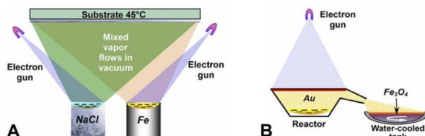
Fig. 1 Schematic representation of  $\text{Fe}_3\text{O}_4$ -Au MNC synthesis *via* EB-PVD: (A) iron and sodium chloride are vaporized by an electron beam, then the vapors condense on a cooled substrate, forming iron nanoparticles embedded in NaCl matrix; (B) following oxidation the nanoparticles are coated with gold evaporated from a reactor.
