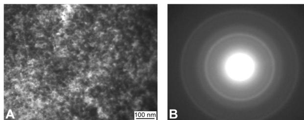
Fig. 2 TEM image (A) and electron pattern (B) of  $\text{Fe}_3\text{O}_4$  nanoparticles synthesized using EB-PVD.
