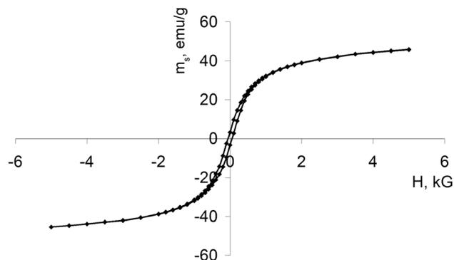
Fig. 6 Magnetic hysteresis loop measured for Fe<sub>3</sub>O<sub>4</sub>-Au MNC at room temperature.
