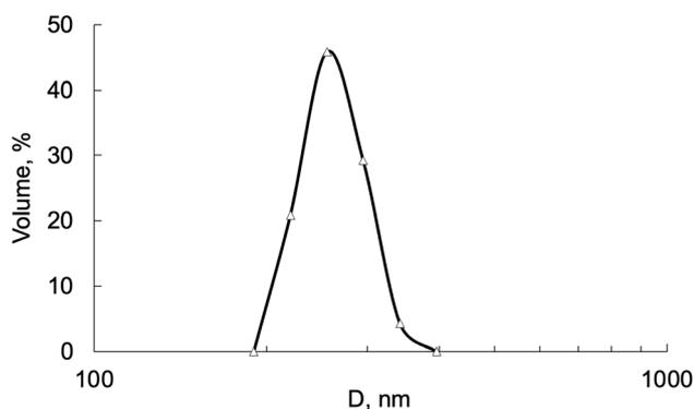
Fig. 5 Hydrodynamic size ( $D$ ) of Fe<sub>3</sub>O<sub>4</sub>-Au MNC in aqueous solution.
