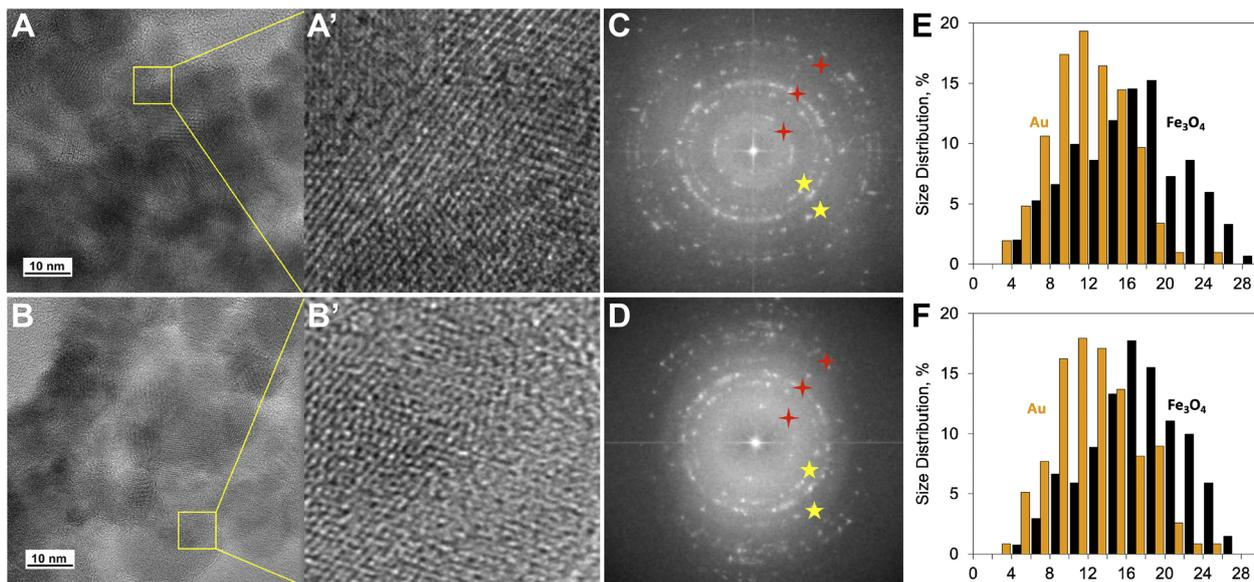
Fig. 4 TEM, FFT images and size distributions of Fe<sub>3</sub>O<sub>4</sub>-Au MNC before (A, A', C and E) and after DOX loading (B, B', D and F): TEM images with increasing magnification from A to A' and B to B'; FFT images (C and D): yellow marks correspond to the contributions of gold and red marks correspond to the contributions of Fe<sub>3</sub>O<sub>4</sub>; size (nm) distributions (E and F) of Au and Fe<sub>3</sub>O<sub>4</sub> nanoparticles comprising MNC.
