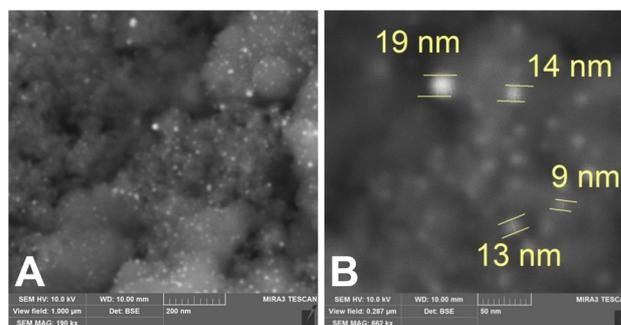
Fig. 3 SEM images with increasing magnification from (A) and (B) of  $\text{Fe}_3\text{O}_4$ -Au MNC: EB-PVD formed island structures of gold (bright spots) on the surface of magnetite nanoparticles (dark spots).
