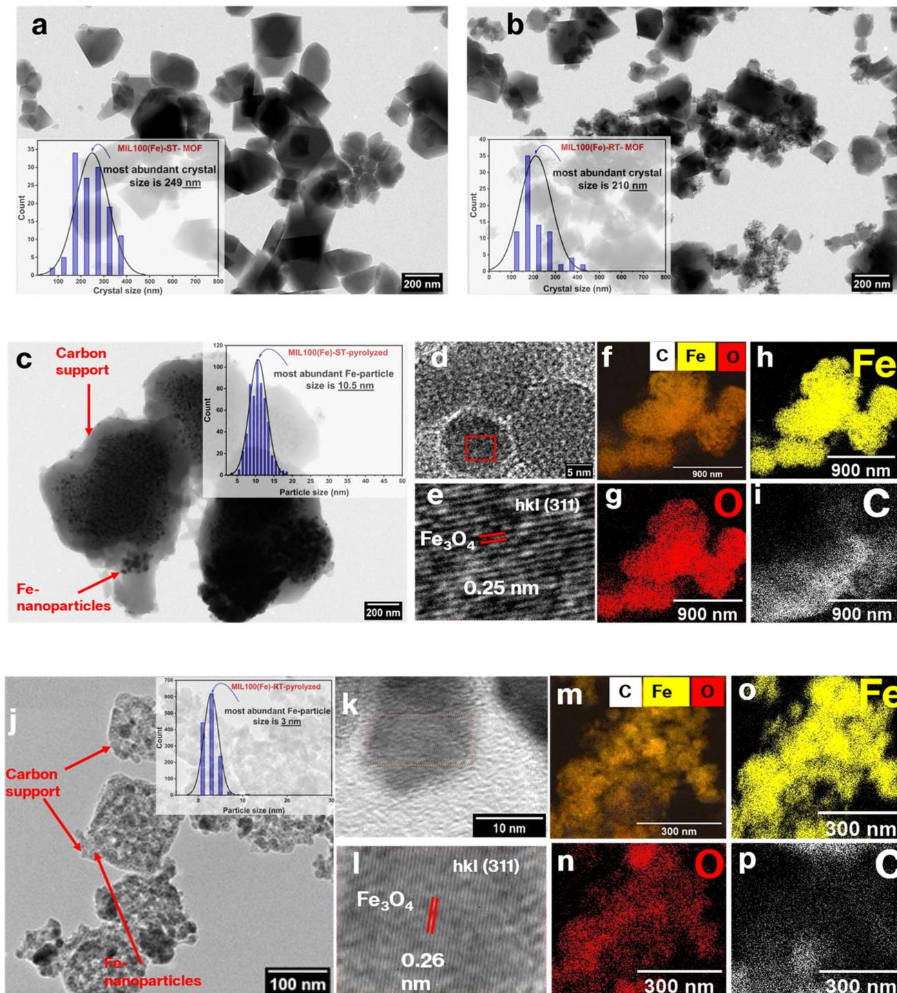
**Fig. 1** TEM images for (a) MIL-100(Fe)-ST (inset crystal size distribution (CSD)), (b) MIL-100(Fe)-RT (inset crystal size distribution (CSD)), (c) MIL-100(Fe)-ST after pyrolysis, and PSD (inset), (d and e) HRTEM images, and (f–i) TEM-EDS elemental mapping; (j) TEM image for MIL-100(Fe)-RT after pyrolysis, and PSD (inset), (k and l) HRTEM images, and (m–p) TEM-EDS elemental mapping.
