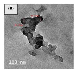
Fig. 7 TEM of (a) poly(MMA/DMAEMA/CHAA) and (b) poly(MMA/DMAEMA/CHAA)-TiO<sub>2</sub>.
