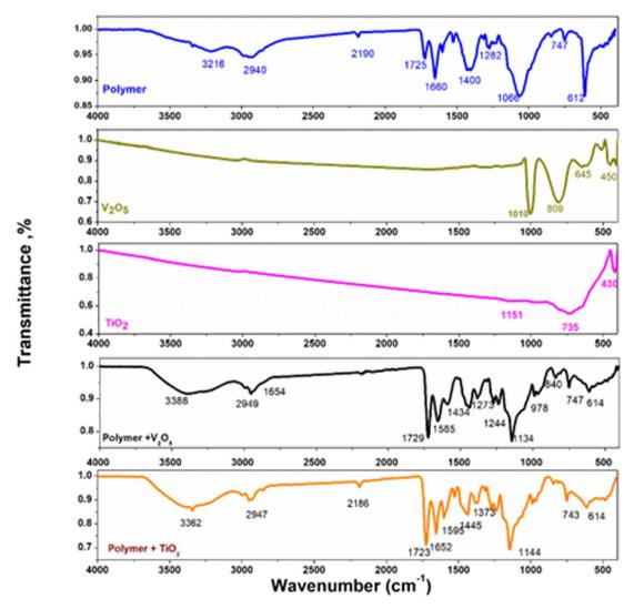
Fig. 4 FTIR spectra of V<sub>2</sub>O<sub>5</sub>, TiO<sub>2</sub>, poly(MMA/DMAEMA/CHAA), poly(MMA/DMAEMA/CHAA)-V<sub>2</sub>O<sub>5</sub>, and poly(MMA/DMAEMA/CHAA)-TiO<sub>2</sub>.
