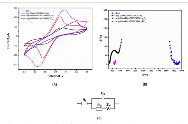
Fig. 10 (A) CV and (B) EIS data for the different poly(MMA/DMAEMA/CHAA)-MOs nanocomposites performance using a mixture solution of 5 mM ferri/ferrocyanide and 0.1 M KCl and scan rate of 50 mV s $^{-1}$ . (C) Fitting circuit.
