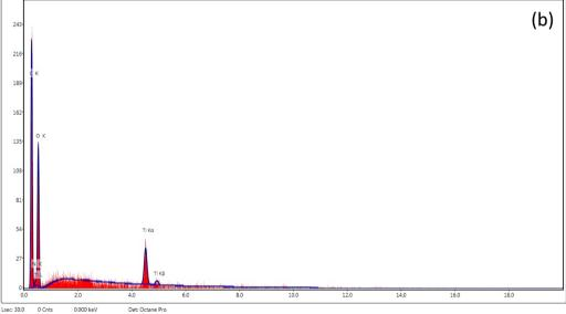
$\mbox{Fig. 8} \ \ \mbox{SEM and EDX of (a) poly(MMA/DMAEMA/CHAA) and (b) poly(MMA/DMAEMA/CHAA)-TiO_2. } \\$
