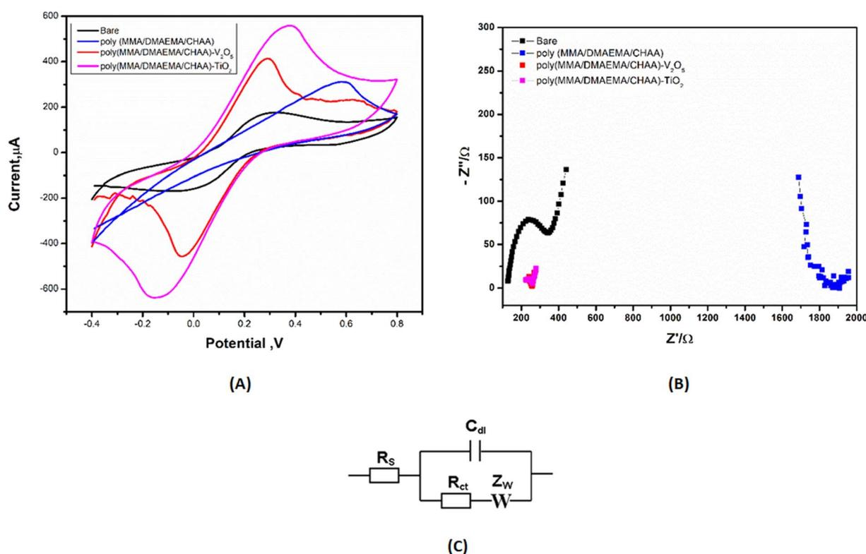
Fig. 10 (A) CV and (B) EIS data for the different poly(MMA/DMAEMA/CHAA)-MOs nanocomposites performance using a mixture solution of 5 mM ferri/ferrocyanide and 0.1 M KCl and scan rate of 50 mV s<sup>-1</sup>. (C) Fitting circuit.
