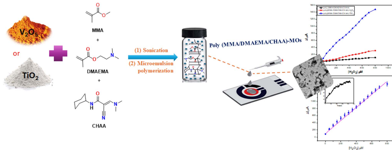
Fig. 1 Synthesis of poly(MMA/DMAEMA/CHAA) nanospheres and nanocomposites via microemulsion polymerization and poly(MMA/DMAEMA/CHAA)-MOs screen-printed electrode modification method with their electrochemical measurements.
