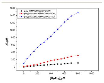
Fig. 14 Amperometry calibration curves of different poly(MMA/DMAEMA/CHAA)-MOs nanocomposites in PBS buffer pH 7.0 and different concentrations of  $\rm H_2O_2$ .
