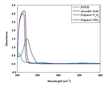
Fig. 9 Typical absorption spectra of 100  $\mu$ M of the DPPH radical alone and in the presence of a 200  $\mu$ M concentration of polymer +  $V_2O_5$ , polymer +  $TiO_2$  and vitamin C.
