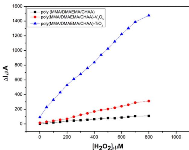
Fig. 14 Amperometry calibration curves of different poly(MMA/DMAEMA/CHAA)-MOs nanocomposites in PBS buffer pH 7.0 and different concentrations of H<sub>2</sub>O<sub>2</sub>.
