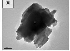
Fig. 2 TEM images of (A) TiO<sub>2</sub> and (B) V<sub>2</sub>O<sub>5</sub> nanoparticles.
