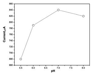
Fig. 13 The pH effect on poly(MMA/DMAEMA/CHAA)-TiO<sub>2</sub> sensor performance towards peroxide oxidation response.
