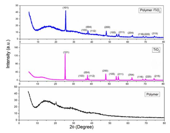
Fig. 6 XRD of pure poly(MMA/DMAEMA/CHAA), TiO<sub>2</sub>, and (MMA/DMAEMA/CHAA)-TiO<sub>2</sub>.
