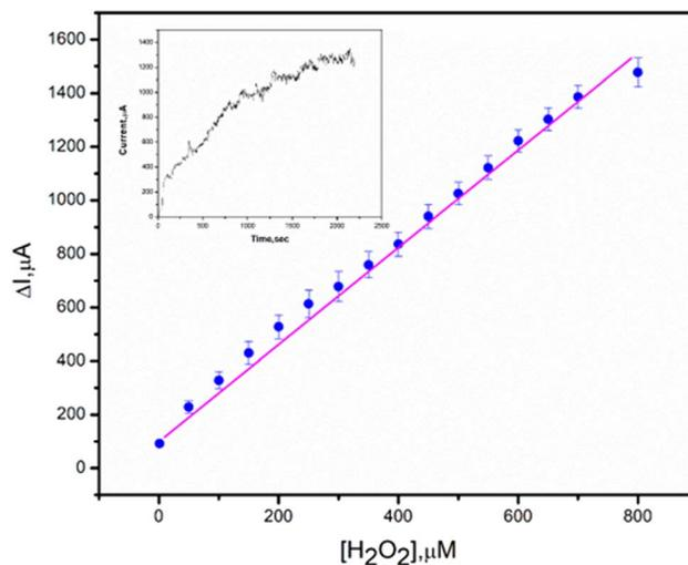
Fig. 15 The corresponding calibration curve of poly(MMA/DMAEMA/CHAA)-TiO<sub>2</sub> modified SPE toward H<sub>2</sub>O<sub>2</sub> response.
