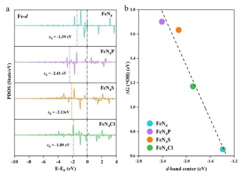
Fig. 7 (a) Projected density of states of the Fe atom on FeN<sub>4</sub>, FeN<sub>4</sub>P, FeN<sub>4</sub>S and FeN<sub>4</sub>Cl, and their corresponding d-band centers. (b) Relationship between the d-band center of the Fe atom in FeN<sub>4</sub>, FeN<sub>4</sub>P, FeN<sub>4</sub>S and FeN<sub>4</sub>Cl and  $\Delta G(^*OH)$ .
