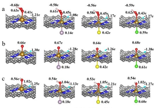
Fig. 6 Bader charge analysis of FeN<sub>4</sub>, FeN<sub>4</sub>P, FeN<sub>4</sub>S and FeN<sub>4</sub>Cl for (a) \*OOH, (b) \*O and (c) \*OH, respectively.
