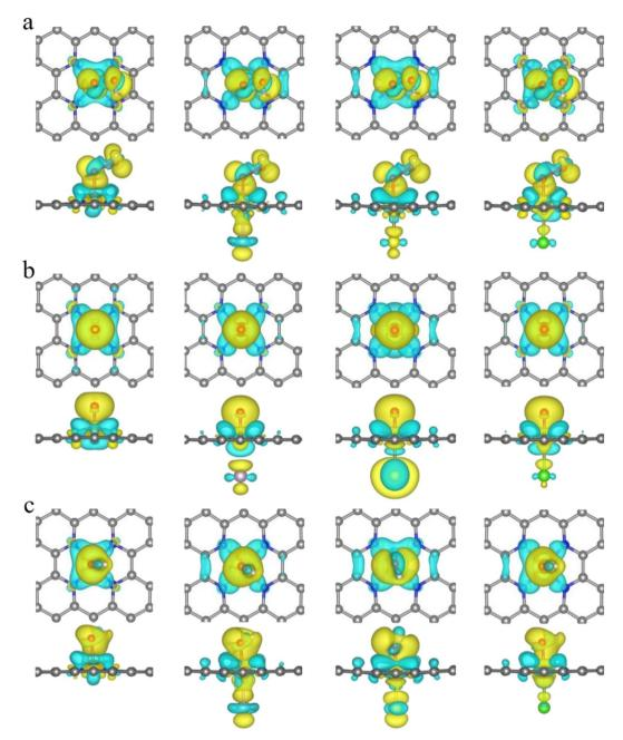
Fig. 5 The differential charge density of FeN<sub>4</sub>, FeN<sub>4</sub>P, FeN<sub>4</sub>S and FeN<sub>4</sub>Cl for (a) \*OOH, (b) \*O and (c) \*OH, respectively. The isosurface is 0.002 e  $Å^{-3}$ .
