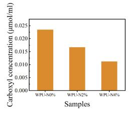
Fig. 9 Carboxylic group concentration on the surface of WPU-N0%, WPU-N2% and WPU-N4% coating ( $2.5 \text{ cm} \times 2.5 \text{ cm}$ ).
