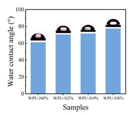
Fig. 8 Contact angle of WPU coatings with different nerol contents.
