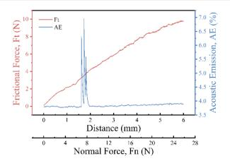
Fig. 12 Scratch test result of WPU-N2% coating.
