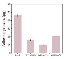
Fig. 10 Amount of bovine serum albumin adhering to the surface of WPU-N0%, WPU-N2% and WPU-N4% coating (1 cm  $\times$  1 cm).
