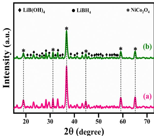
Fig. 10 XRD patterns of  $\text{LiBH}_4 + 75\% \text{NiCo}_2\text{O}_4$  (a) after hydrogenation ( $150^\circ\text{C}$  for 30 min under 10 bar) and (b) after dehydrogenation at  $275^\circ\text{C}$ .
