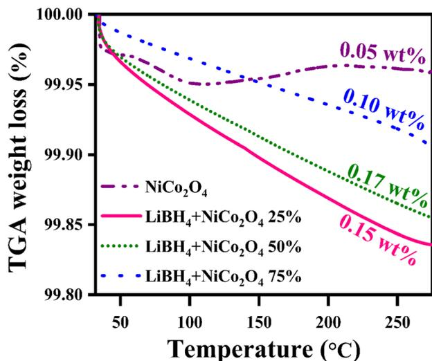
Fig. 4 Thermal stability curves of  $\text{NiCo}_2\text{O}_4$ ,  $\text{LiBH}_4 + 25\% \text{NiCo}_2\text{O}_4$ ,  $\text{LiBH}_4 + 50\% \text{NiCo}_2\text{O}_4$  and  $\text{LiBH}_4 + 75\% \text{NiCo}_2\text{O}_4$  systems before hydrogenation.
