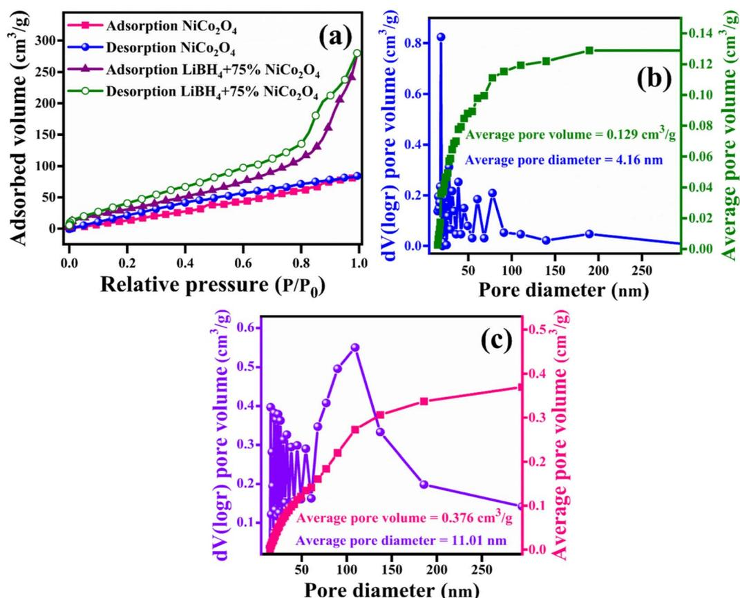
Fig. 8 (a) Nitrogen adsorption/desorption curves of NiCo $_2$ O $_4$  and LiBH $_4$  + 75% NiCo $_2$ O $_4$ ; BJH pore size distribution curves of (b) NiCo $_2$ O $_4$  and (c) LiBH $_4$  + 75% NiCo $_2$ O $_4$ .
