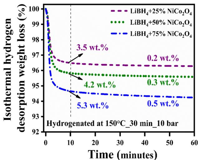
Fig. 6 Isothermal hydrogen desorption curves of LiBH<sub>4</sub> + 25% NiCo<sub>2</sub>O<sub>4</sub>, LiBH<sub>4</sub> + 50% NiCo<sub>2</sub>O<sub>4</sub> and LiBH<sub>4</sub> + 75% NiCo<sub>2</sub>O<sub>4</sub> systems.
