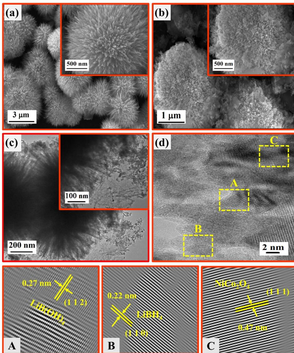
Fig. 7 SEM images of (a) NiCo<sub>2</sub>O<sub>4</sub> and (b) LiBH<sub>4</sub> + 75% NiCo<sub>2</sub>O<sub>4</sub>; (c) TEM images of LiBH<sub>4</sub> + 75% NiCo<sub>2</sub>O<sub>4</sub>; (d) HRTEM images of LiBH<sub>4</sub> + 75% NiCo<sub>2</sub>O<sub>4</sub>.
