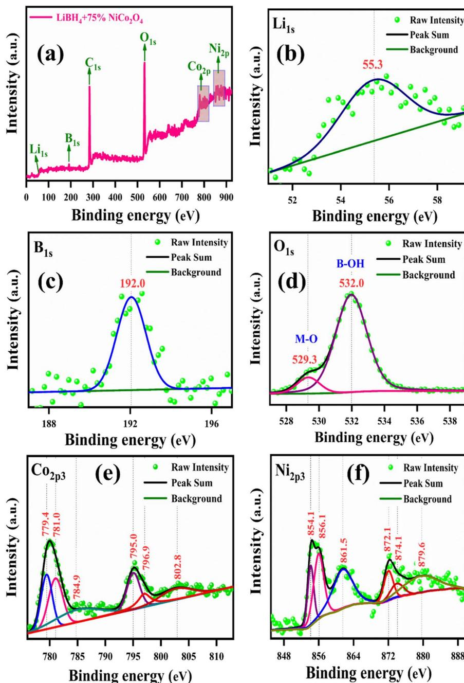
Fig. 9 XPS spectrum of  $\text{LiBH}_4 + 75\% \text{NiCo}_2\text{O}_4$ : (a) survey spectrum, (b) Li 1s, (c) B 1s, (d) O 1s, (e) Co 2p<sub>3</sub>, and (f) Ni 2p<sub>3</sub>.
