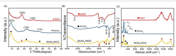
Fig. 2 The PXRD patterns (A), FTIR spectra (B) and Raman spectra (C) of NGO, MoSe<sub>2</sub> and MoSe<sub>2</sub>/NGO materials.
