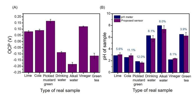
Fig. 7 OCP values of real samples over  $MoSe_2/NGO/SPE$  (A) and the corresponding pH values obtained from the  $MoSe_2/NGO/SPE$  sensor and commercial pH meter (indicated in blue: % difference in pH values between the proposed sensor and commercial pH meter) (B).
