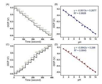
Fig. 5 Open-circuit potential responses of pH 2-14 solutions (A), the corresponding calibration curves (B), open-circuit potential responses of pH 14-2 solutions (C), and the corresponding calibration curves (D) using MoSe<sub>2</sub>/NGO/SPE
