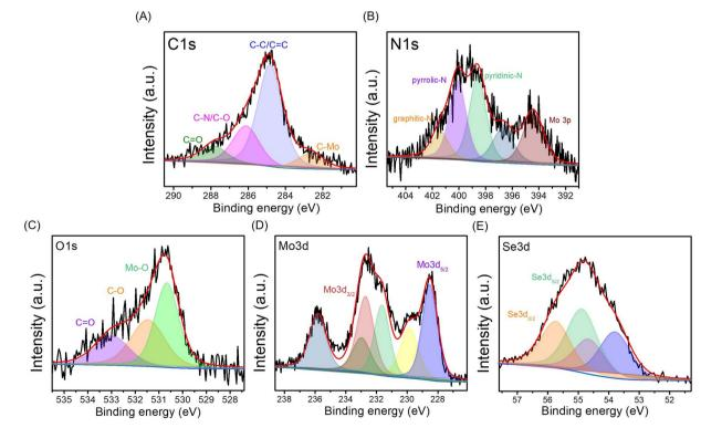
High-resolution XPS spectra of MoSe<sub>2</sub>/NGO: C1s (A), N1s (B), O1s (C), Mo3d (D), and Se3d (E).
