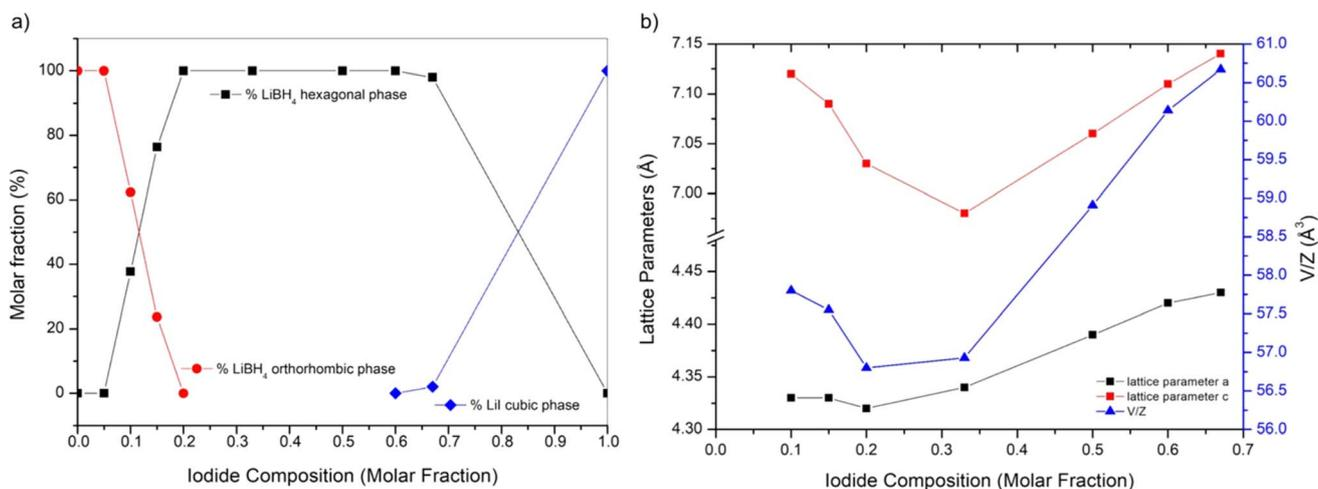
Fig. 2 (a) Phase fraction and (b) lattice parameters and unit volume of the cell ( $V/Z$ ) of the hexagonal phase as a function of the nominal LiI molar fraction for all the synthesized samples. Connecting lines are a guide for the eyes.
