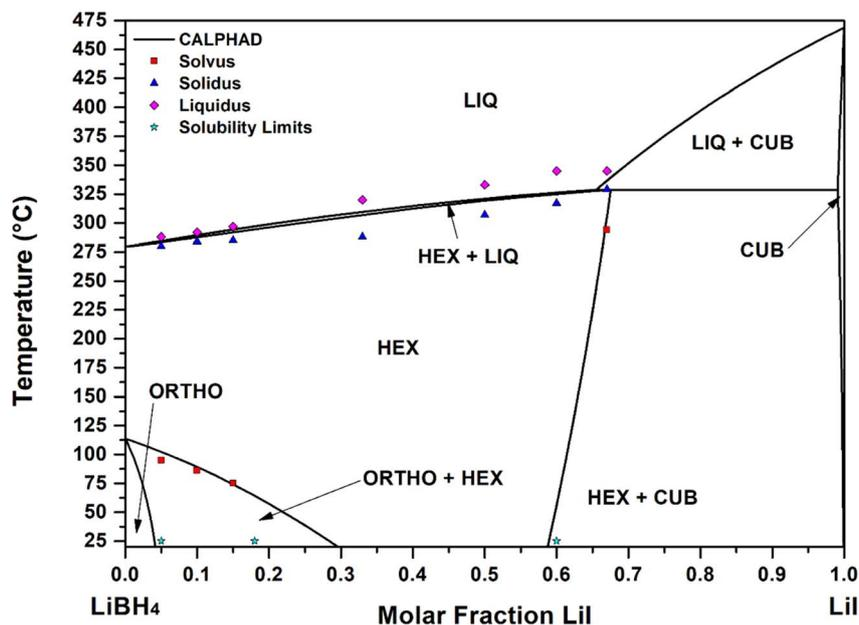
Fig. 5 Lines: assessed phase diagram for the LiBH<sub>4</sub>-LiI system. Experimental temperature data determined in this work from DSC are reported as: red squares (solvus), blue triangles (solidus), pink diamonds (liquidus). Light blue stars indicate solubility limits determined in this work by XRD and Rietveld analysis at room temperature.
