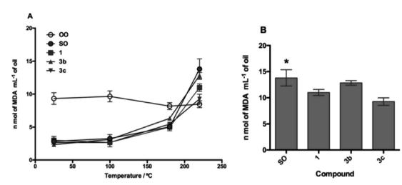
Fig. 7 Lipid peroxidation process in the presence of compound 1 and its derivatives 3b and 3c. (A) Lipid oxidation process as temperature increases and (B) statistical analysis of the oxidation process at 220 °C. SO: sunflower oil. \*p < 0.05 with respect to 3c.
