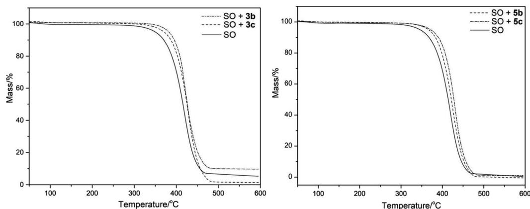
Fig. 4 TG curves of sunflower oil (SO) and SO supplemented with the *O*-alkyl derivatives **3b–c** and **5b–c**.
