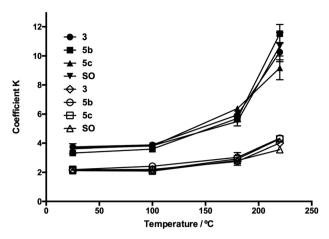
Fig. 6 Evolution of extinction coefficients  $K_{232}$  and  $K_{270}$  through the heating process for oil additives **5b** and **5c**. SO: sunflower oil without additive,  $K_{232}$ : symbol in black, and  $K_{270}$ : symbol in white.
