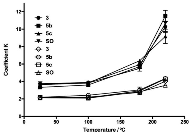
Fig. 6 Evolution of extinction coefficients  $K_{232}$  and  $K_{270}$  through the heating process for oil additives 5b and 5c. SO: sunflower oil without additive,  $K_{232}$ : symbol in black, and  $K_{270}$ : symbol in white.
