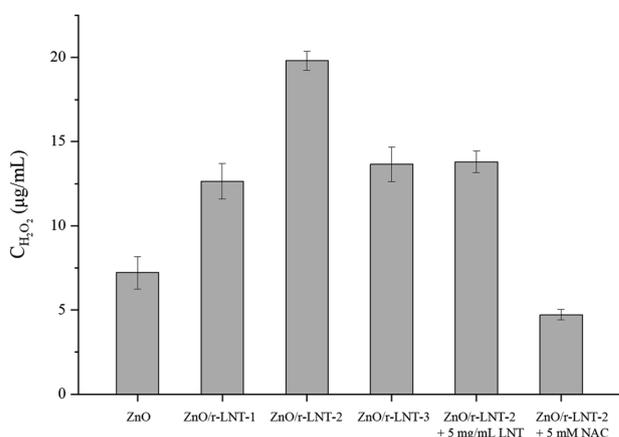
Fig. 8  $\text{H}_2\text{O}_2$  produced by ZnO, ZnO/r-LNT-1, ZnO/r-LNT-2, ZnO/r-LNT-3, and ZnO/r-LNT-2 +  $5 \text{ mg mL}^{-1}$  LNT suspensions. All sample contains  $2 \text{ mg mL}^{-1}$  ZnO. All particles in the suspension were removed after standing for 12 h at room temperature.
