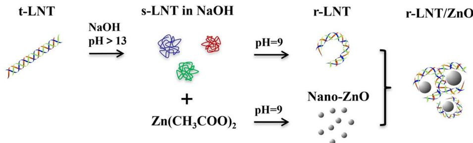
Fig. 1 Scheme of ZnO NPs dispersion by r-LNT.
