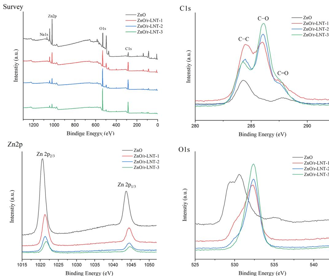
Fig. 6 XPS spectra of ZnO, ZnO/r-LNT-1, ZnO/r-LNT-2 and ZnO/r-LNT-3.
