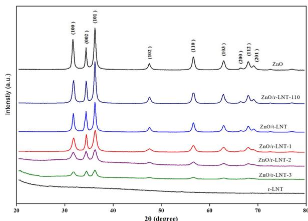
Fig. 3 XRD spectra of ZnO, LNT and their nanocomposites.
