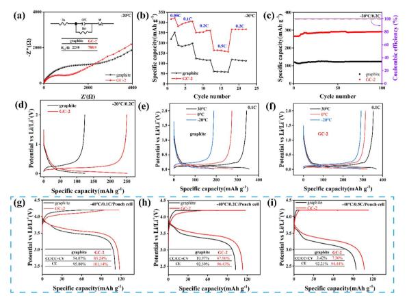
Fig. 5 Low-temperature performance of pristine graphite and GC-2. Half cells of (a) EIS Nyquist curves at -20 °C, (b) rate performance from 0.05 to 0.5C (1C = 370 mA h  $g^{-1}$ ), (c) cycle performance at 0.2C, (d) charge/discharge curves at 0.2C, (e and f) charge/discharge curves at 0.1C from 30 °C to -20 °C. Pouch cell charge/discharge curves under -40 °C at (g) 0.1C, (h) 0.2C, (i) 0.5C.
