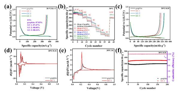
Fig. 2 Electrochemical performance of pristine graphite and GCs: (a) the first charge/discharge curves and initial coulombic efficiency at 0.1C; (b) rate performance from 0.1 to 5C ( $1C = 370 \text{ mA h g}^{-1}$ ); (c) charge/discharge curves at 0.5C; dQ/dV curves of pristine graphite and GC-2 at 0.1C (d) and 3C (e); (f) cycle performance of pristine graphite and GC-2 at 0.5C.
