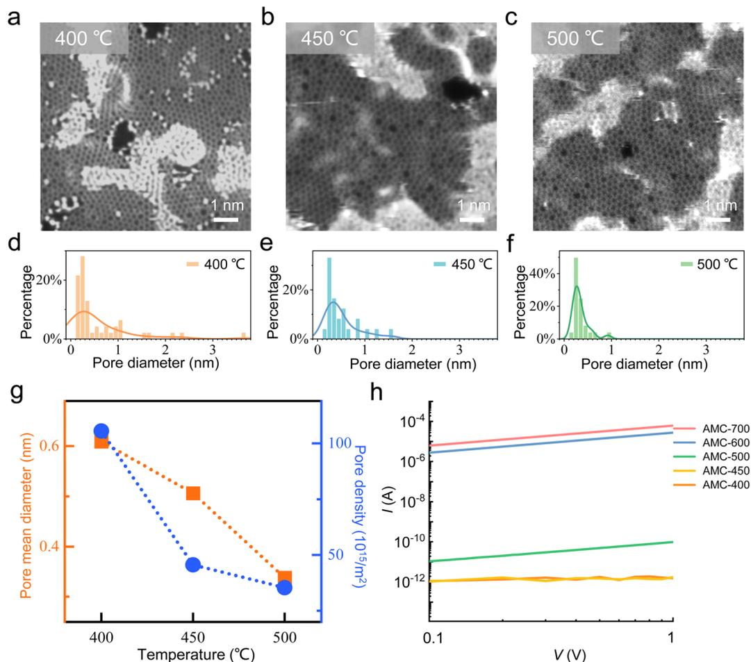
Fig. 2 Atomic-scale STEM and electrical characterization of AMC obtained at different temperatures. (a–c) Representative STEM images of AMC-400 (a), AMC-450 (b) and AMC-500 (c). (d–f) Histogram of pore diameters in AMC-400 (d), AMC-450 (e) and AMC-500 (f) with fitted curves. (g) Statistics of pore mean diameters and pore densities of AMC. (h) Results from two-terminal electrical  $I$ – $V$  measurements on AMC.
