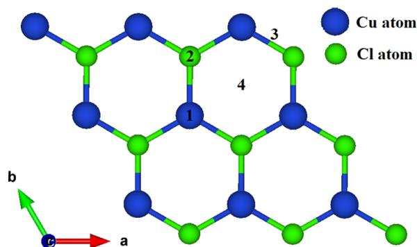
Fig. 1 CuCl ML, with different adsorption sites.
