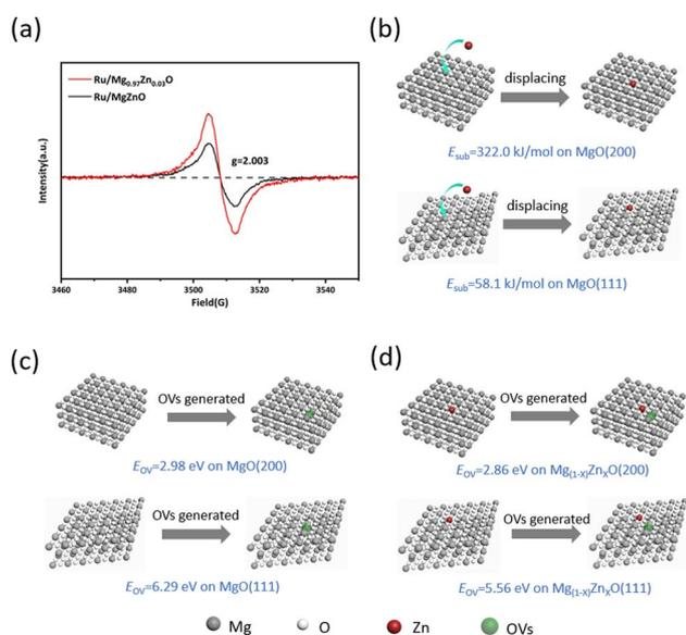
Fig. 4 (a) EPR spectra of Ru/Mg<sub>(1-x)</sub>Zn<sub>x</sub>O and Ru/MgO catalysts (b) substitution energy ( $E_{\text{sub}}$ ) on different crystal faces of MgO. (c) Oxygen vacancy formation energy ( $E_{\text{OV}}$ ) before Zn doping on (200) and (111) crystal planes of MgO. (d) Oxygen vacancy formation energy ( $E_{\text{OV}}$ ) after Zn doping on (200) and (111) crystal planes of Mg<sub>(1-x)</sub>Zn<sub>x</sub>O.
