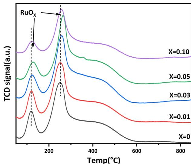
Fig. 9  $\text{H}_2$ -TPR curves of Ru/Ba- $\text{Mg}_{(1-x)}\text{Zn}_x\text{O}$  catalysts.
