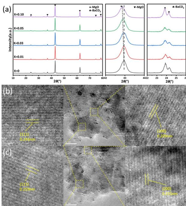
Fig. 2 (a) XRD results of Ru/Ba–Mg<sub>(1–X)</sub>Zn<sub>X</sub>O catalysts and amplification of the position at 42–44° and 22–26° of  $2\theta$  angle. (b) Lattice spacing of the (200) and (111) crystal planes of Ru/Ba–MgO (c) lattice spacing of the (200) and (111) crystal planes of Ru/Ba–Mg<sub>0.97</sub>Zn<sub>0.03</sub>O catalysts.
