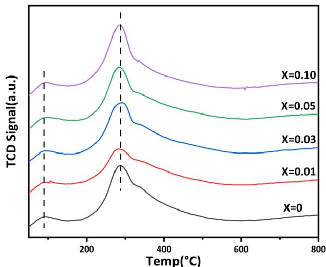
Fig. 8  $CO_2$ -TPD curve of Ru/Ba–Mg<sub>(1-x)</sub>Zn<sub>x</sub>O catalysts.
