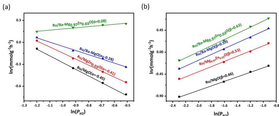
Fig. 7 (a) Reaction orders of  $H_2$  for Ru/MgO, Ru/Ba–MgO, Ru/Mg<sub>0.97</sub>Zn<sub>0.03</sub>O and Ru/Ba–Mg<sub>0.97</sub>Zn<sub>0.03</sub>O catalysts. (b) Reaction orders of  $N_2$  for Ru/MgO, Ru/Ba–MgO, Ru/Mg<sub>0.97</sub>Zn<sub>0.03</sub>O and Ru/Ba–Mg<sub>0.97</sub>Zn<sub>0.03</sub>O catalysts.
