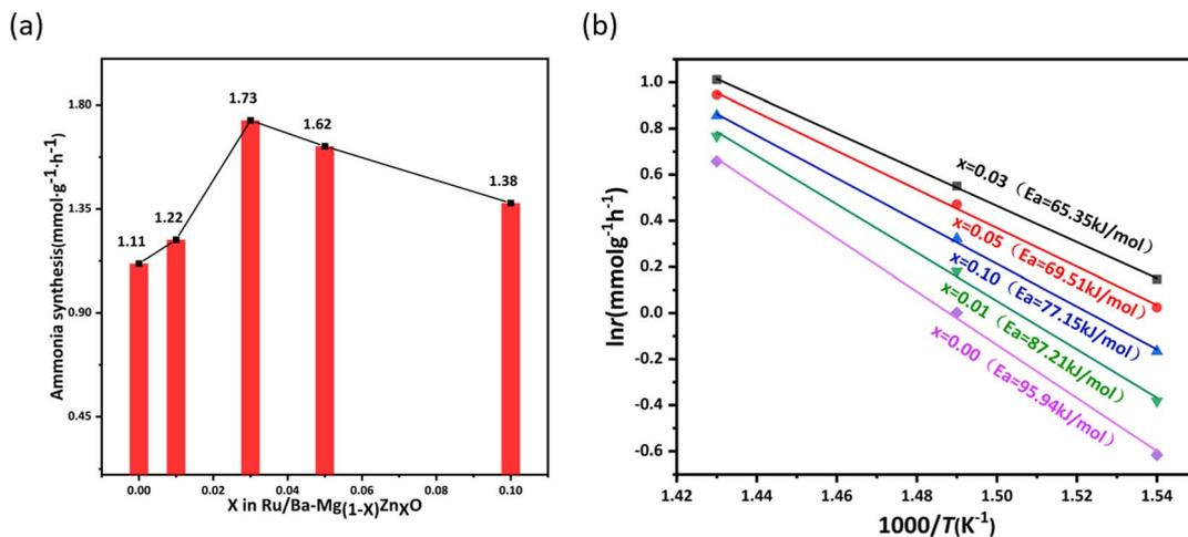
Fig. 1 (a) Ammonia synthesis rate of Ru/Ba–Mg<sub>(1–X)</sub>Zn<sub>X</sub>O catalysts. Test condition: 0.2 MPa, 400 °C, 18 000 h<sup>–1</sup>. (b) E<sub>a</sub> of Ru/Ba–Mg<sub>(1–X)</sub>Zn<sub>X</sub>O catalysts (375–425 °C).
