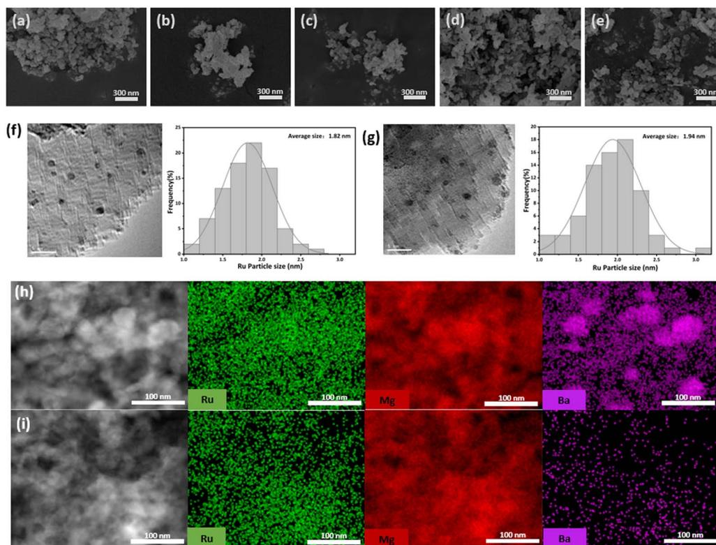
**Fig. 3** SEM of Ru/Ba-Mg<sub>(1-x)</sub>Zn<sub>x</sub>O catalysts (a)  $X = 0$  (b)  $X = 0.01$  (c)  $X = 0.03$  (d)  $X = 0.05$  (e)  $X = 0.10$ . (f) Size distribution of Ru nanoparticles in Ru/Ba-MgO catalyst. (g) Size distribution of Ru nanoparticles in Ru/Ba-Mg<sub>0.97</sub>Zn<sub>0.03</sub>O catalyst. (h) TEM-Mapping of Ru/Ba-MgO catalyst. (i) TEM-Mapping of Ru/Ba-Mg<sub>0.97</sub>Zn<sub>0.03</sub>O catalyst.
