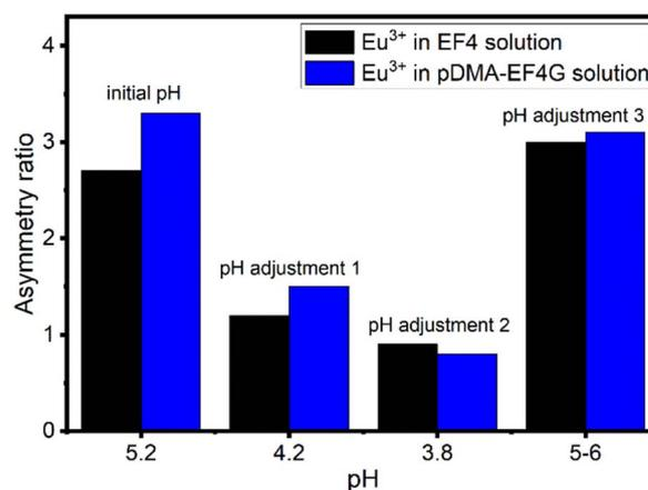
Fig. 5 The change in asymmetry ratio of  $\text{Eu}^{3+}$  in EF4/pDMA-EF4G solution at different pH. Black:  $\text{Eu}^{3+}$  in EF4 solution, blue:  $\text{Eu}^{3+}$  in pDMA-EF4G solution. Asymmetry ratio  $< 1$  indicates the free  $\text{Eu}^{3+}$  aquo ion.
