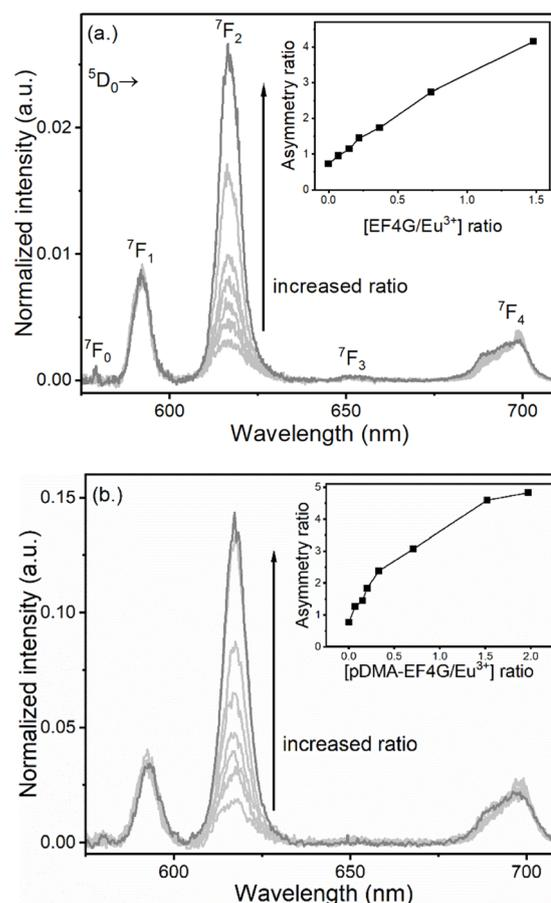
Fig. 2 Luminescence spectra of  $\text{Eu}^{3+}$  at pH 5 taken at gate delay  $10 \mu\text{s}$  with increasing concentration of (a) EF4G and (b) pDMA-EF4G. The complexation of  $\text{Eu}^{3+}$  with the peptide indicated by the increase of the  $^5\text{D}_0 \rightarrow ^7\text{F}_2$ , “the hypersensitive” peak intensity; inset: asymmetry ratio.
