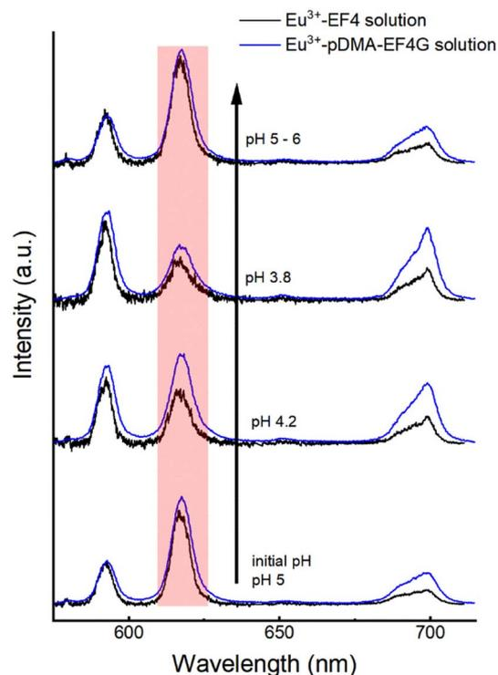
Fig. 4 Spectral change of  $\text{Eu}^{3+}$ -EF4/pDMA-EF4G (1 : 1 molar ratio) luminescence upon alteration of the pH. The change in intensity of  ${}^5\text{D}_0 \rightarrow {}^7\text{F}_2$  (hypersensitive) peak indicates the binding reversibility: at pH 4.2 the intensity started to decrease, at pH 3.8 the luminescence spectrum resembles largely the  $\text{Eu}^{3+}$  aquo ion upon increasing the pH above 5 the luminescence of the peptide complex is observed again.
