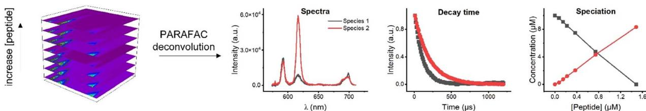
Fig. 1 Four-dimensional data cube in PARAFAC analysis consists of emission wavelength, intensity, and time as *x*-, *y*-, *z*- axis, respectively, with different peptide concentration as the fourth axis. PARAFAC deconvolution yielded information regarding the species.
