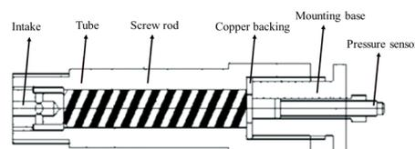
Fig. 3 Test device of quasi-static pressure.
