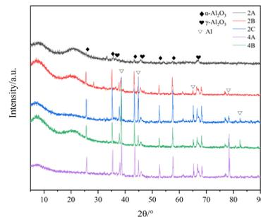
Fig. 8 XRD patterns of the residue after detonation.
