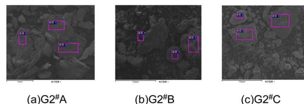
Fig. 10 SEM images for the EDS test of solid residue products after detonation: (a) G2<sup>#</sup>A; (b) G2<sup>#</sup>B; (c) G2<sup>#</sup>C.
