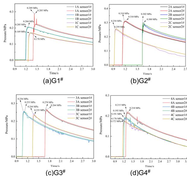
Fig. 4 Explosion pressure–time curves of the samples: (a) G1<sup>#</sup>; (b) G2<sup>#</sup>; (c) G3<sup>#</sup>; (d) G4<sup>#</sup>.
