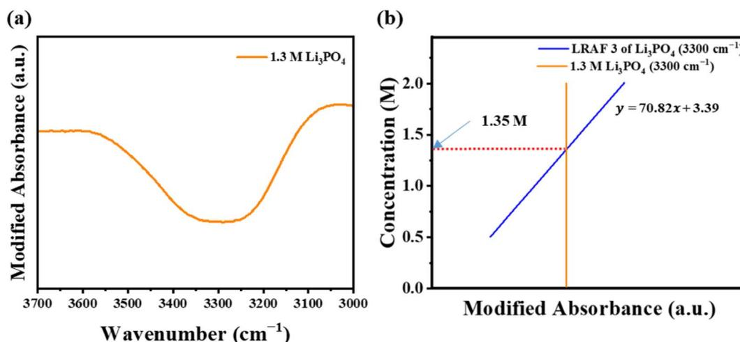
Fig. 4 (a) Absorbance of the 1.3 M Li<sub>3</sub>PO<sub>4</sub> (LiOH + H<sub>3</sub>PO<sub>4</sub>) solution in the O–H stretching band range (3000–3700 cm<sup>−1</sup>). (b) Molarity calculated by LRAF 3 for Li<sub>3</sub>PO<sub>4</sub> (3300 cm<sup>−1</sup>)
