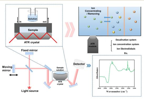
Fig. 1 Schematic diagrams of ATR-FTIR measurement principle and its application to various agueous ion systems.
