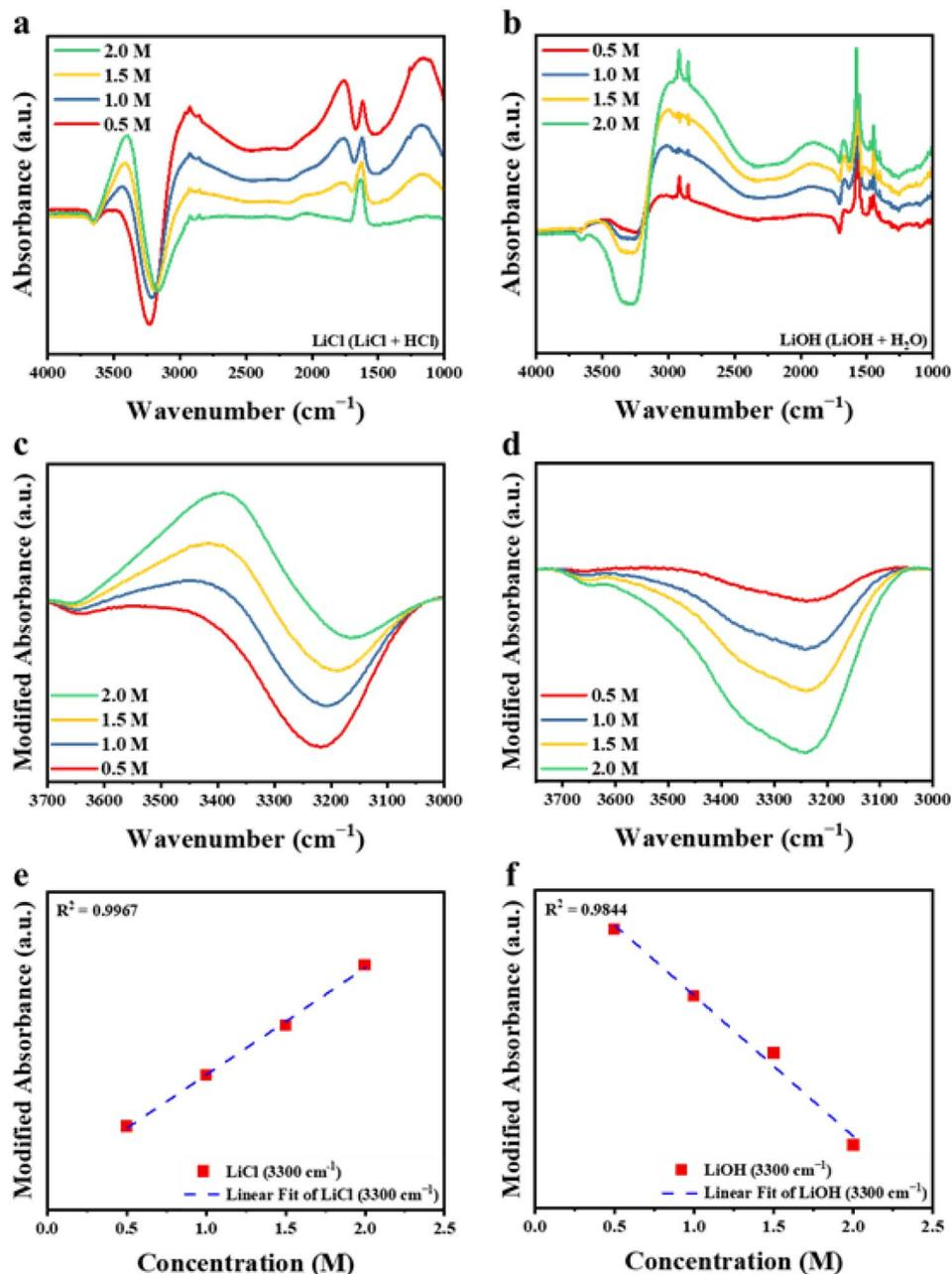
Fig. 2 (a and b) ATR-FTIR absorbance of the LiCl (LiCl + HCl) and LiOH (LiOH + H<sub>2</sub>O) solutions depending on the molarity of the cation. (c and d) Differences in the absorbance of the O–H stretching band at 3300 cm<sup>-1</sup> in LiCl (LiCl + HCl) and LiOH (LiOH + H<sub>2</sub>O) solutions based on cation (Li<sup>+</sup>) molarity. (e and f) Linear regression analysis function graphs of absorbance based on the cation molarity in (c and d).
