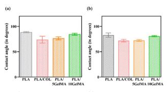
Fig. 6 Contact angle measurement (a) cementum layer for PLA, PLA/COL, PLA/5 GelMA and PLA/10 GelMA (b) bone layer for PLA, PLA/COL, PLA/5 GelMA and PLA/10 GelMA.
