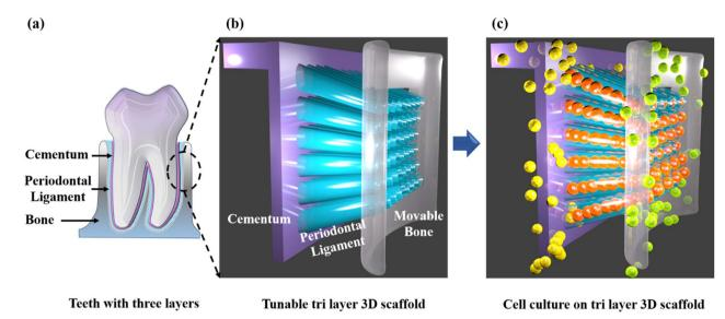
Fig. 1 Schematic of direction-oriented fiber guiding with tunable tri-layer-3D scaffold (a) teeth with three layers (b) fabricated direction-oriented fiber guiding with tunable tri layer -3D scaffold (c) cell culture on direction-oriented fiber guiding tri layer 3D scaffold.
