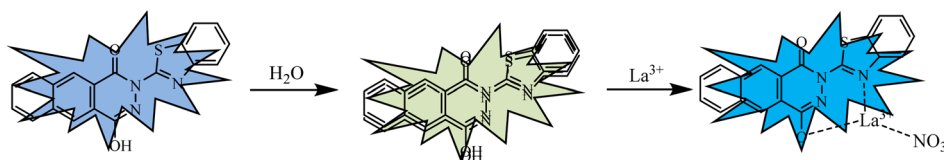
Scheme 2 Plausible sensing mechanism of probe N for La 3+ .
