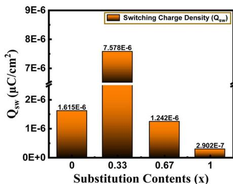
Fig. 11 Switching charge density of the Ba<sub>1-x</sub>Sr<sub>x</sub>NiO<sub>3</sub> samples at different substitution contents (x).
