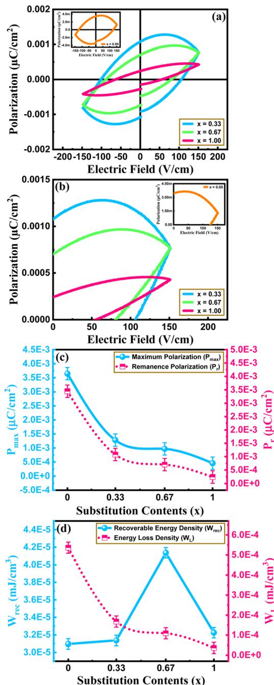
Fig. 7 (a) Polarization versus electric field hysteresis loops, (b) charge-discharge regions of the  $P$ - $E$  loops, (c) variation in maximum and remanent polarization by changing the substitution content, and (d) change in recoverable energy density and energy loss density with increases in Sr-content in the Ba<sub>1-x</sub>Sr<sub>x</sub>NiO<sub>3</sub> samples with  $x = 0.00, 0.33, 0.67, \text{ and } 1.00$ .
