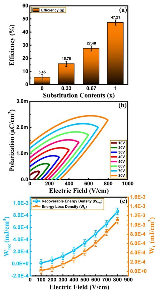
Fig. 8 (a) Percentage efficiency in all the  $\text{Ba}_{1-x}\text{Sr}_x\text{NiO}_3$  samples, (b) charge-discharge curves, and (c) variation in recoverable energy density and energy loss density at different potentials in the pure  $\text{SrNiO}_3$  sample.
