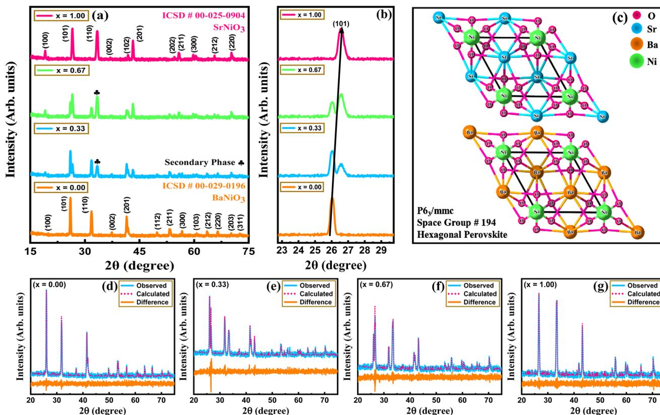
Fig. 2 (a) Indexed XRD patterns of the Ba<sub>1-x</sub>Sr<sub>x</sub>NiO<sub>3</sub> samples with  $x = 0.00, 0.33, 0.67$ , and  $1.00$ , (b) shifting of the (101) peak towards higher angles, (c) crystal structure of BaNiO<sub>3</sub> and SrNiO<sub>3</sub>, and (d)–(g) Rietveld's refined XRD patterns of the Ba<sub>1-x</sub>Sr<sub>x</sub>NiO<sub>3</sub> samples with  $x = 0.00, 0.33, 0.67$ , and  $1.00$ .
