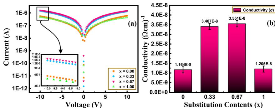
**Fig. 9** (a)  $I$ - $V$  characteristics curves and (b) the conductivity of the  $Ba_{1-x}Sr_xNiO_3$  samples with  $x = 0.00, 0.33, 0.67,$  and  $1.00$ .
