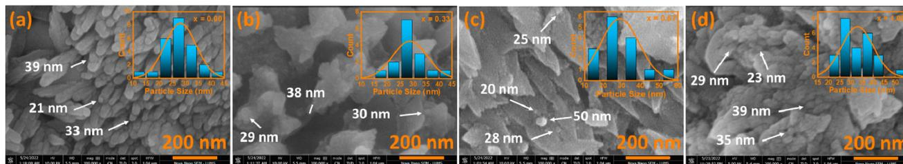
Fig. 5 SEM images of the  $\text{Ba}_{1-x}\text{Sr}_x\text{NiO}_3$  samples with  $x =$  (a) 0.00, (b) 0.33, (c) 0.67, and (d) 1.00 captured at a magnification of 200 000 $\times$ . The relevant in-sets show respective grain size distributions.
