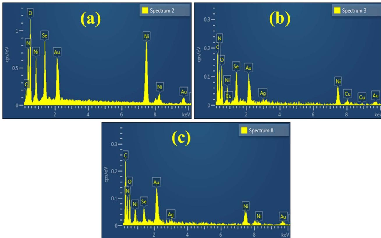
Fig. 6 Elemental composition of (a) NiSe, (b) Ag/C<sub>3</sub>N<sub>4</sub>-doped NiSe, and (c) C<sub>3</sub>N<sub>4</sub>/Ag-doped NiSe.
