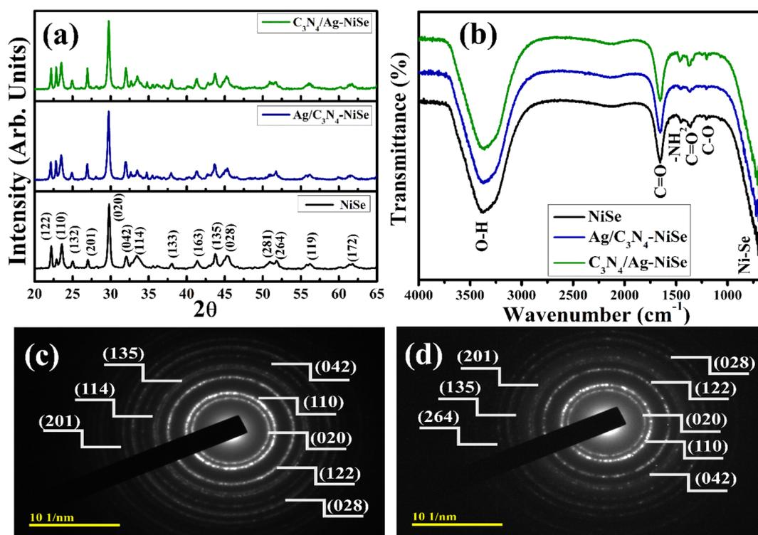
Fig. 2 (a) X-ray diffraction pattern, (b) FTIR spectra and (c and d) SAED images of NiSe and Ag/C<sub>3</sub>N<sub>4</sub>-doped NiSe.
