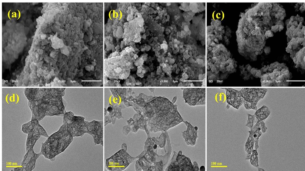
Fig. 4 Structure and surface morphology of NiSe, Ag/C<sub>3</sub>N<sub>4</sub> and C<sub>3</sub>N<sub>4</sub>/Ag-doped NiSe (a–c) SEM analysis and (d–f) TEM analysis.
