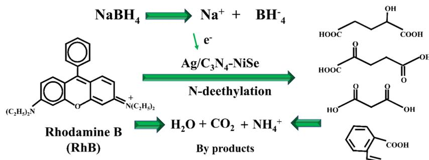
Fig. 9 Schematic illustration of the catalytic mechanism for the degradation of the RhB dye.
