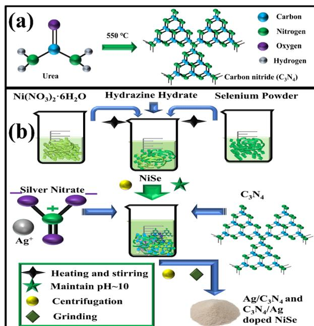
Fig. 1 Schematic of the synthesis of (a) C<sub>3</sub>N<sub>4</sub>, (b) NiSe, Ag/C<sub>3</sub>N<sub>4</sub> and C<sub>3</sub>N<sub>4</sub>/Ag-doped NiSe.
