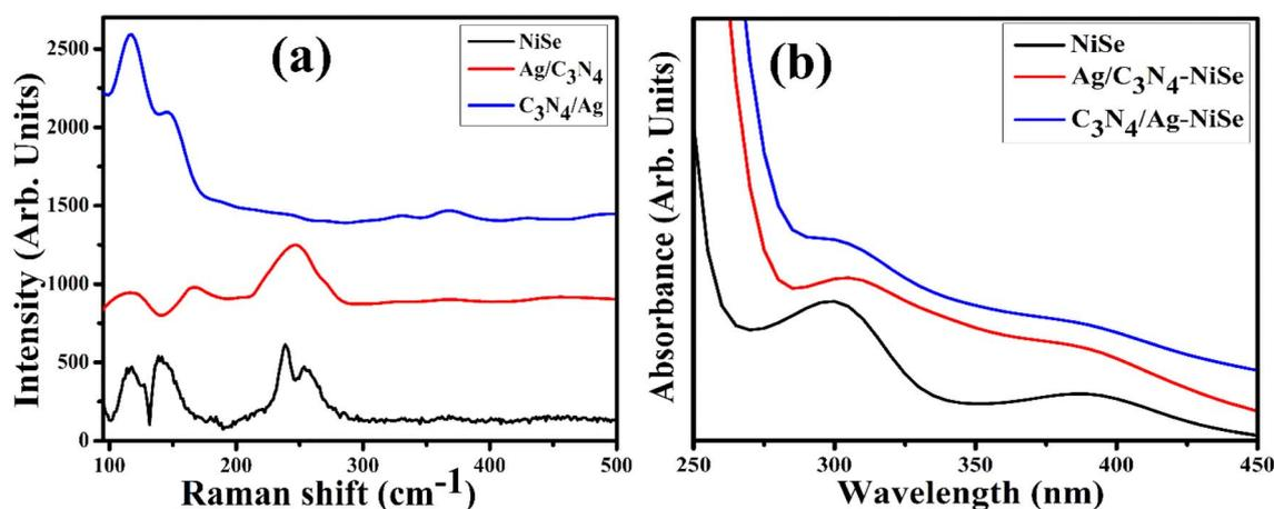
Fig. 3 (a) Raman spectra and (b) optical absorbance spectra of NiSe, Ag/C<sub>3</sub>N<sub>4</sub> and C<sub>3</sub>N<sub>4</sub>/Ag-doped NiSe NWs.
