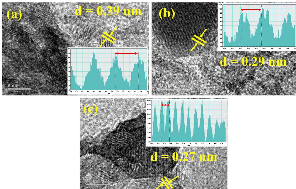
Fig. 5 The interlayer *d*-spacing of synthesized NWs (a) NiSe, (b) Ag/C<sub>3</sub>N<sub>4</sub>-doped NiSe, and (c) C<sub>3</sub>N<sub>4</sub>/Ag-doped NiSe.
