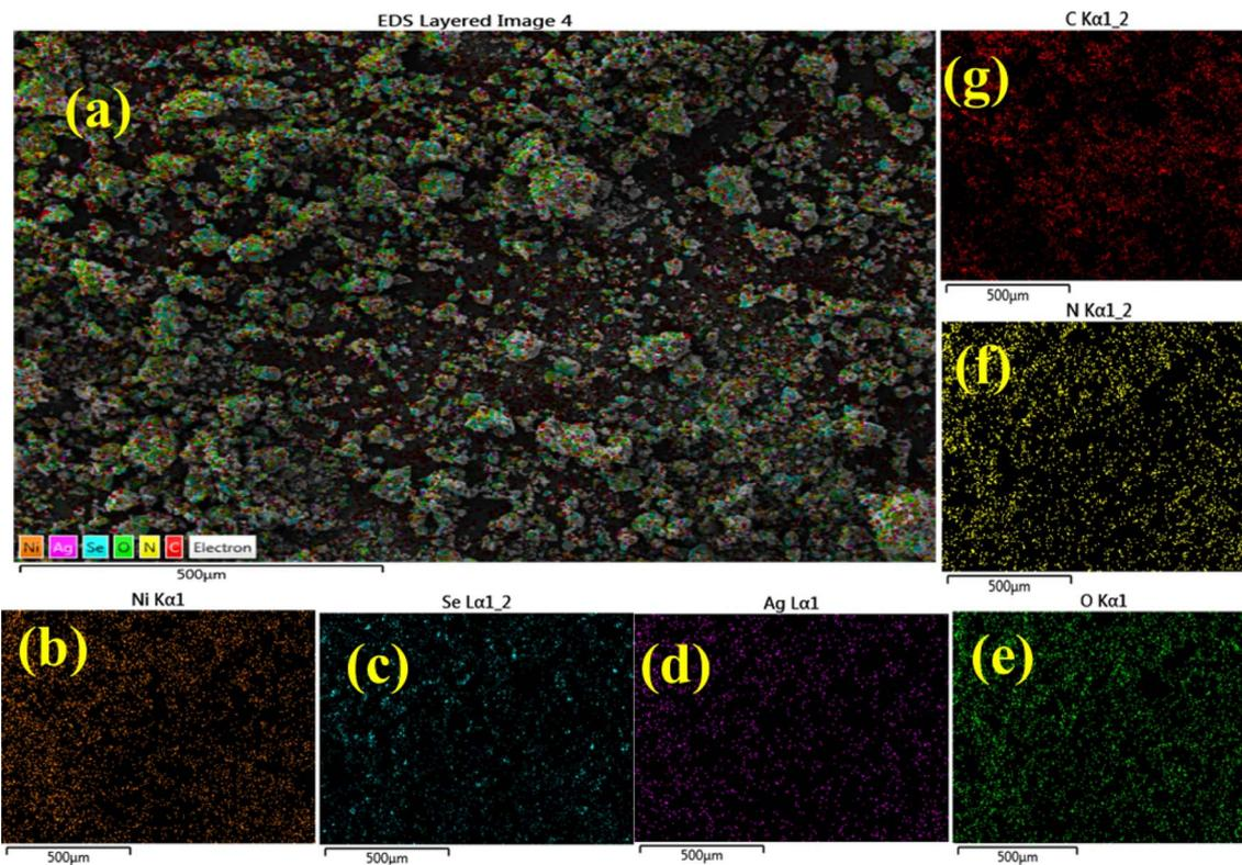
Fig. 7 Elemental mapping analysis of (a) C<sub>3</sub>N<sub>4</sub>/Ag-doped NiSe (b) Ni, (c) Se, (d) Ag, (e) O, (f) N, and (g) C atoms.
