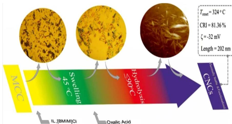
Fig. 3 Preparation of cellulose nanocrystals by ionic liquid (IL)-mediated technique.<sup>29</sup>
