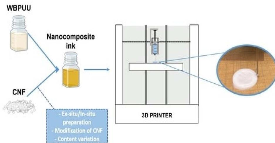
Fig. 6 Three-dimensional-printed waterborne polyurethane-urea-based nanocomposite inks.<sup>56</sup>
