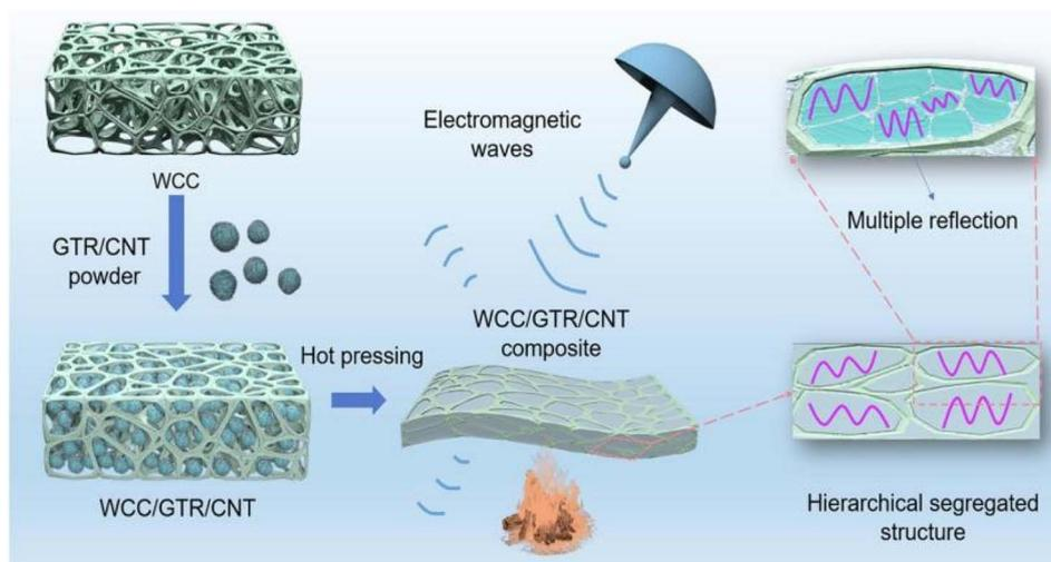
Fig. 8 Schematic diagram of the preparation of WCC/GTR/CNT composites.<sup>66</sup>
