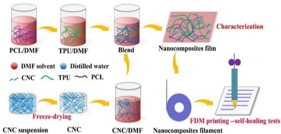
Fig. 7 TPU/PCL/CNC nanocomposite preparation and FDM printing process.<sup>60</sup>
