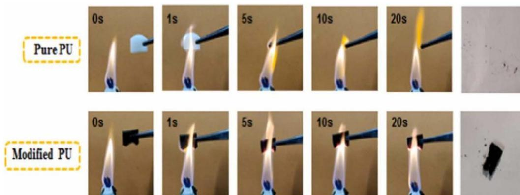
Fig. 9 Combustion process of a PU sponge.<sup>69</sup>
