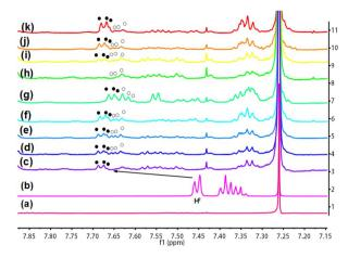
Fig. 2 Partial NMR spectra of MA with various enantiomeric excess (a) L-TPP-P, (b)  $\pm$ MA, (c) R/S = 5:0, (d) R/S = 5:1, (e) R/S = 5:2, (f) R/S = 5:3, (g) R/S = 5:5, (h) R/S = 0:5, (i) R/S = 1:5, (j) R/S = 2:5, (k) R/S = 3:5 in the presence of L-TPP-P in CDCl<sub>3</sub>. ( $\blacksquare$  represents the R configuration).
