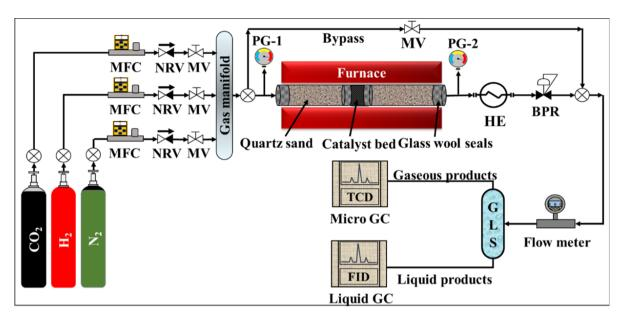
Fig. 1 Schematic of experimental setup used in present study. (MFC: mass flow controller, NRV: non-return valve, MV: manual valve, HE: heat exchanger, BPR: back pressure regulator, GLS: gas-liquid separator, GC: gas chromatography.)
