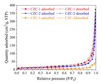
Fig. 3 N<sub>2</sub> adsorption-desorption isotherms of CZC catalysts.
