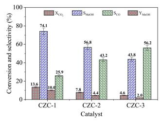
Fig. 8 Catalytic performance of CZC catalysts (experimental conditions: T = 225 °C, P = 30 bar, WHSV = 6000 cm<sup>3</sup> ( $g_{cat}$  h)<sup>-1</sup>, and  $H_2/CO_2$  mole ratio = 3).
