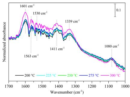
Fig. 10 Influence of temperature on in situ DRIFTS spectra during CO<sub>2</sub> hydrogenation over CZC-1 catalyst under 1 bar pressure.
