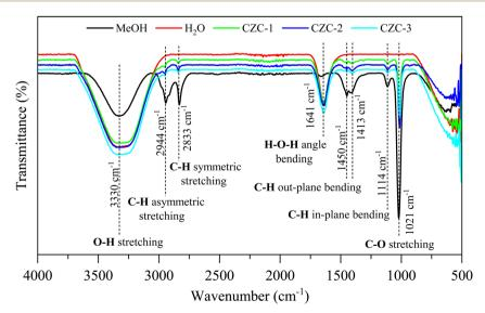
Fig. 7 FTIR spectra of liquid products.
