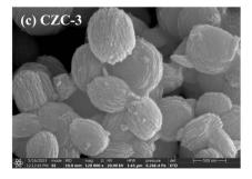
Fig. 4 SEM micrographs of CZC catalysts.
