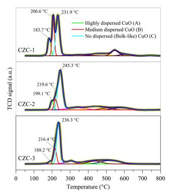
Fig. 6 H<sub>2</sub>-TPR profiles of CZC catalysts
