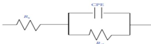
Fig. 4 Electrical circuit equivalent at the carbon steel/HCl electrolyte contact.
