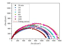
Fig. 10 Nyquist diagram obtained at different immersion times for compound  ${\bf 4}.$
