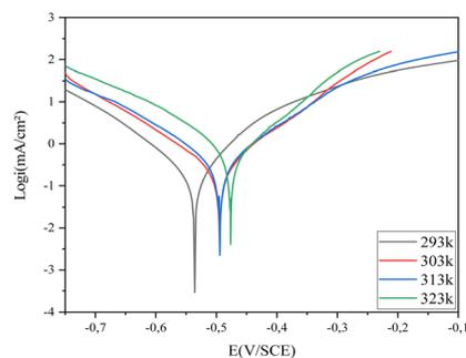
Fig. 6 Polarisation curves for Blank at different temperatures.
