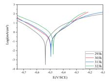
Polarisation curves for Blank at different temperatures
