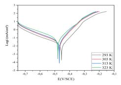
Polarisation curves for compound 4 at different temperatures.
