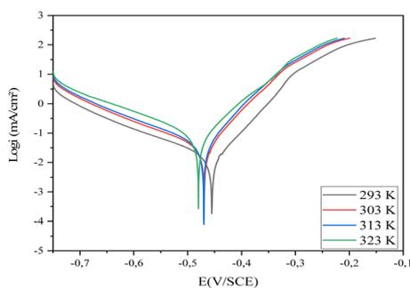
Fig. 5 Polarisation curves for compound 4 at different temperatures.
