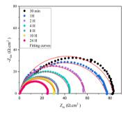
Fig. 11 Nyquist diagram obtained at different immersion times for Blank.
