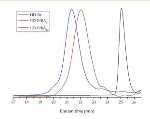
Fig. 3  $\,$  GPC chromatograms of HD-Br, HD-PtBA  $_{\!8}$  and HD-PtBA  $_{\!12}$  with THF as the eluent.
