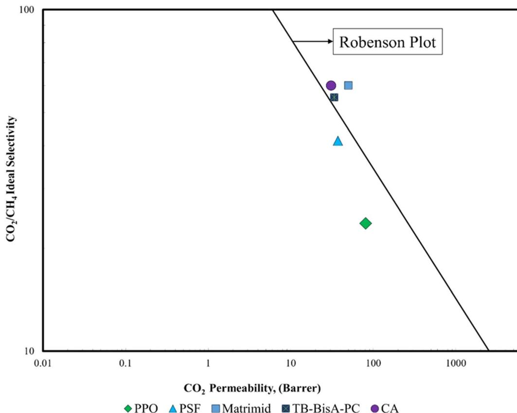
Fig. 2 Robeson plot for different polymers.<sup>39</sup>
