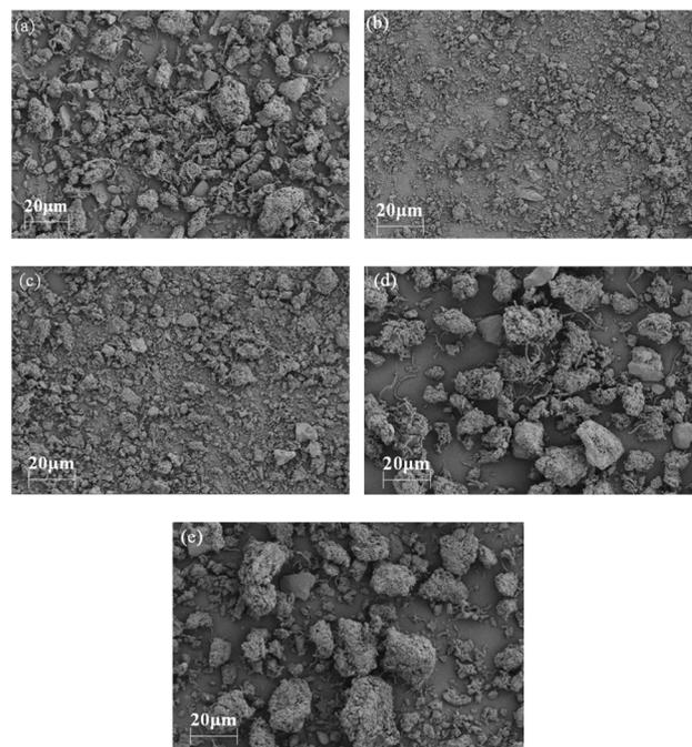
Fig. 7 Changes in sludge morphology under various conditions: (a) original sludge, (b) PDMDAAC alone, (c) HCl alone, (d) FeCl<sub>3</sub> alone, and (e) PDMDAAC + FeCl<sub>3</sub> + HCl.
