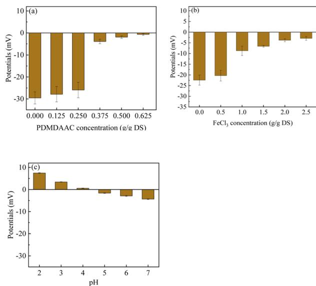
Fig. 6 Variation in zeta potential under different conditions: (a) FeCl<sub>3</sub> dosage of 2.0 g g<sup>-1</sup> DS; (b) PDMDAAC dosage of 0.375 g g<sup>-1</sup> DS; (c) PDMDAAC and FeCl<sub>3</sub> dosages of 0.375 and 2.0 g g<sup>-1</sup> DS, respectively.
