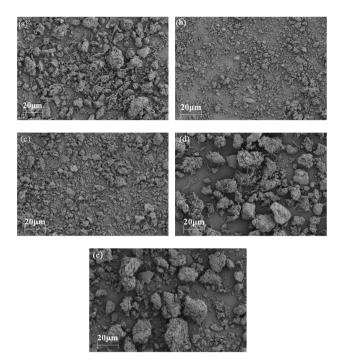
Fig. 7 Changes in sludge morphology under various conditions: (a) original sludge, (b) PDMDAAC alone, (c) HCl alone, (d) FeCl<sub>3</sub> alone, and (e) PDMDAAC + FeCl<sub>3</sub> + HCl.
