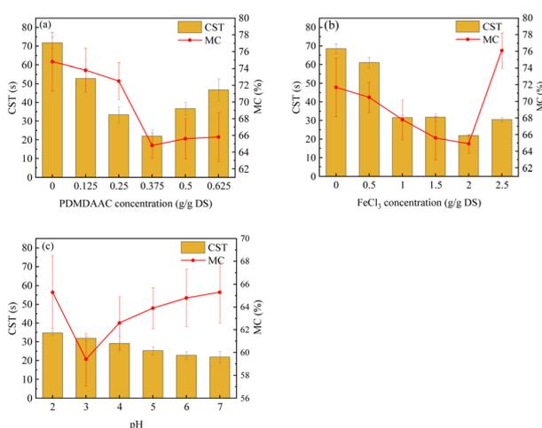
Fig. 1 Variation of sludge MC and CST under different conditions: (a)  $\text{FeCl}_3$  dosage of 2.0  $\text{g g}^{-1}$  DS; (b) PDMDAAC dosage of 0.375  $\text{g g}^{-1}$  DS; (c) PDMDAAC and  $\text{FeCl}_3$  at 0.375 and 2.0  $\text{g g}^{-1}$  DS, respectively.
