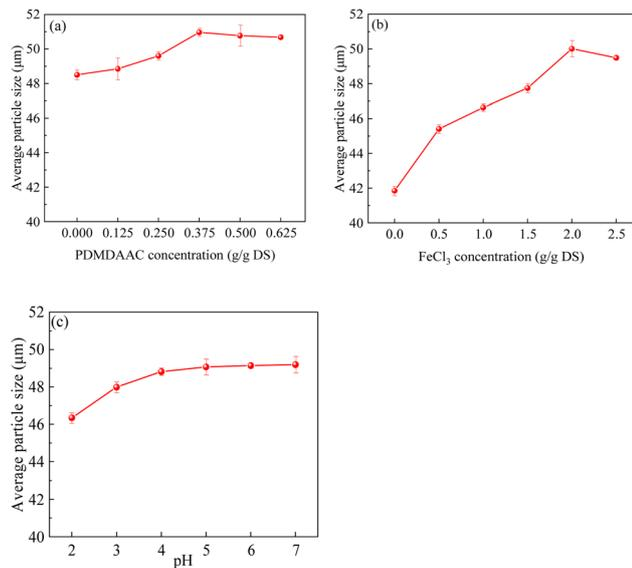
Fig. 5 Variation in sludge particle size under different conditions: (a) FeCl<sub>3</sub> dosage of 2.0 g g<sup>-1</sup> DS; (b) PDMDAAC dosage of 0.375 g g<sup>-1</sup> DS; (c) PDMDAAC and FeCl<sub>3</sub> dosages of 0.375 and 2.0 g g<sup>-1</sup> DS, respectively.
