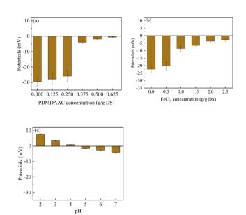
**Fig. 6** Variation in zeta potential under different conditions: (a) FeCl<sub>3</sub> dosage of 2.0 g g<sup>-1</sup> DS; (b) PDMDAAC dosage of 0.375 g g<sup>-1</sup> DS; (c) PDMDAAC and FeCl<sub>3</sub> dosages of 0.375 and 2.0 g g<sup>-1</sup> DS, respectively.
