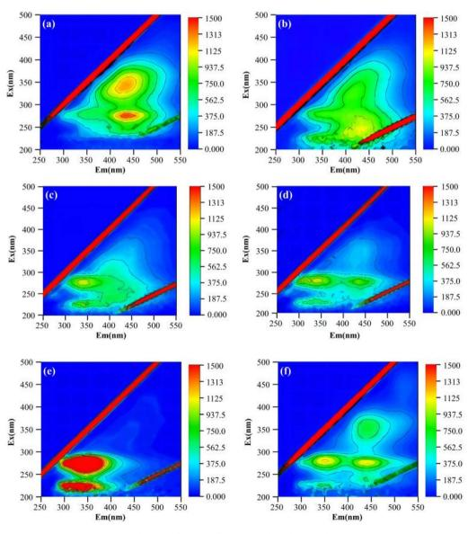
Fig. 3 Variation in fluorescence substances in EPS, where (a, c and e) represent S-EPS, LB-EPS of the original sludge; and (b, d and f) represent S-EPS, LB-EPS, and TB-EPS of the sludge after conditioning.
