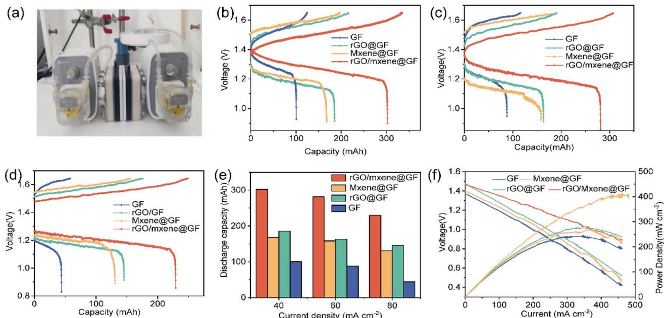
Fig. 8 (a) Picture of battery, charge–discharge curves at (b) 40 mA cm<sup>-2</sup>, (c) 60 mA cm<sup>-2</sup>, and (d) 80 mA cm<sup>-2</sup>, (e) discharge capacities, (f) polarization and power density curves of VRFB.
