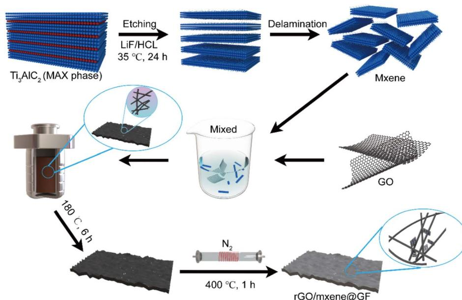
Fig. 1 Schematic diagram of rGO/Mxene@GF synthesis process.
