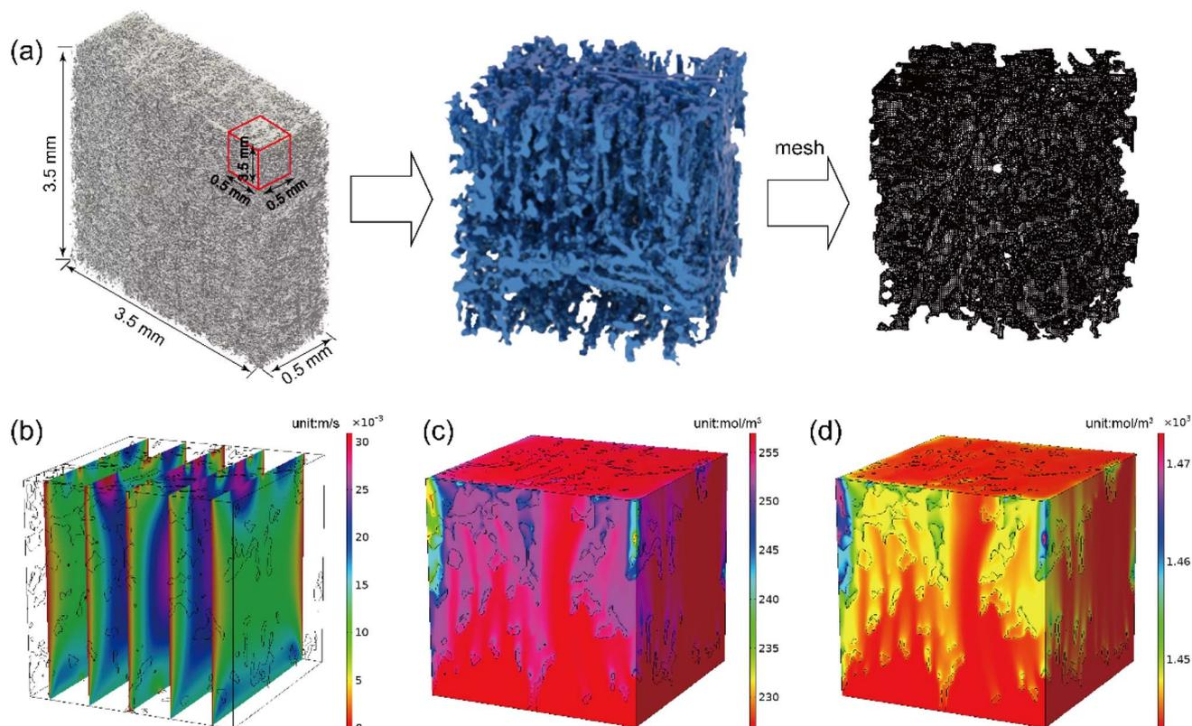
Fig. 7 (a) 3D reconstructed image of the prepared electrode (rGO/Mxene@GF), simulation results of (b) velocity profile, (c)  $\text{V}^{2+}$  concentration and (d)  $\text{V}^{3+}$  concentration distributions in electrode at  $100 \text{ mA cm}^{-2}$ .
