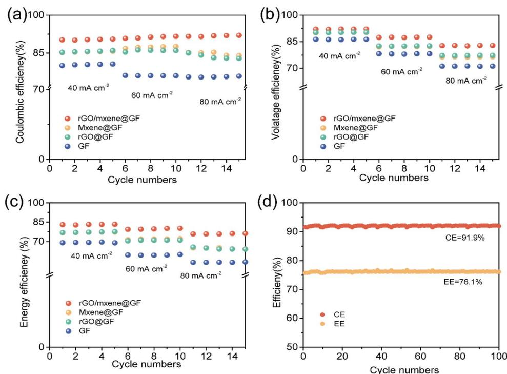
Fig. 9 (a) Coulombic efficiency, (b) voltage efficiency, and (c) energy efficiency of VRFB with different electrodes, (d) cycling performance of VRFB with rGO/Mxene@GF electrode at 80 mA cm<sup>-2</sup>.
