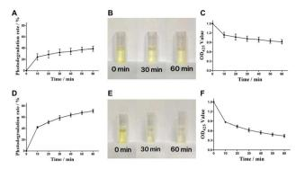
Fig. 2 Light stability of curcumin with red and blue light. (A) Curcumin photodegradation rate in red light. (B) Color change of curcumin in red light. (C)  $OD_{425}$  change of curcumin in red light. (D) Curcumin photodegradation rate in blue light. (E) Color change of curcumin in blue light. (F)  $OD_{425}$  change of curcumin in blue light.
