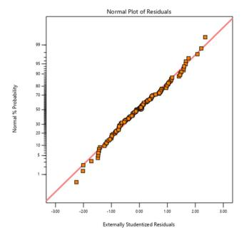
Fig. 4 Plot of residuals and normal probability for MC photodegradation.
