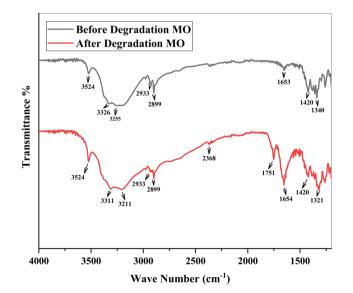
Fig. 6 Shows the FT-IR spectra of methyl orange dye before and after photodegradation.
