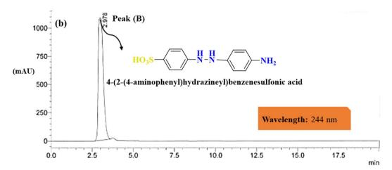
Fig. 7 Illustrates the HPLC spectra of (a) MO before and (b) after photodegradation showing by products peaks.
