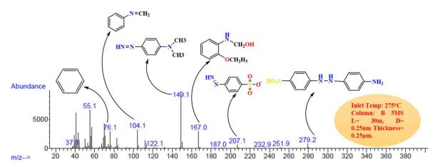
Fig. 8 Shows the GCMS chromatogram of the degradation of MO molecules to smaller fragments.
