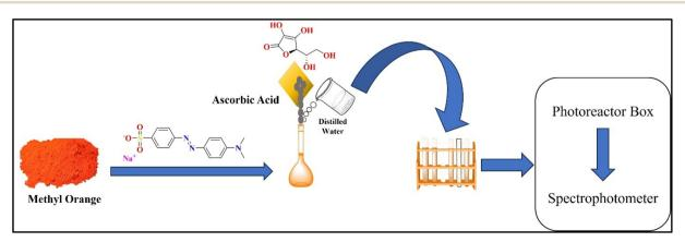
Fig. 1 Illustrates the schematic diagram of the solution preparation and organo-photooxidative activity.
