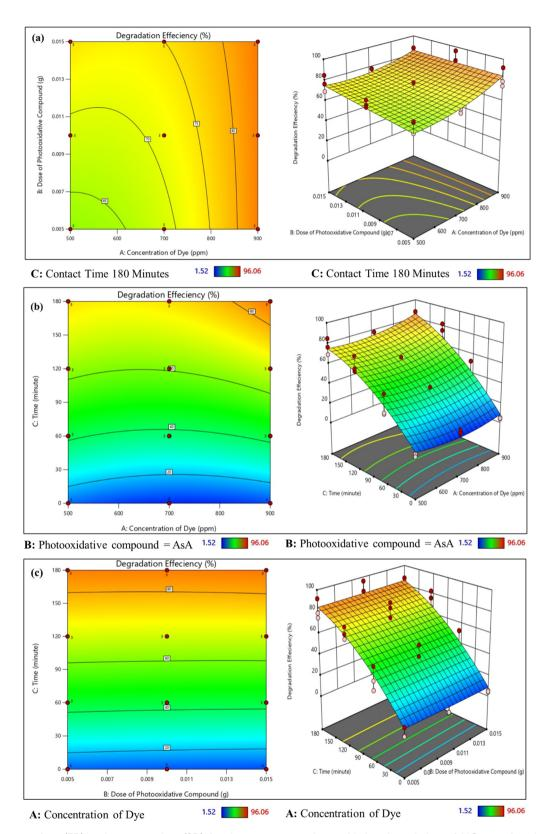
Fig. 3 Response surface (3D) and contour plots (2D) for the percentage photooxidative degradation of MO as a function of (a) A: dye concentration (ppm) and B: dose of photooxidative compound (g) (at contact time = 180 min). (b) A: dye concentration (900 ppm) and C: time (minute): 180 min at dose = 0.015 g, and (c) B: dose of photooxidative compound and C: time (minute) at (dye concentration = 900 ppm and reaction time = 180 min).
