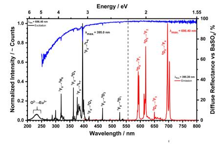
Fig. 4 Diffuse reflectance vs. BaSO<sub>4</sub>, excitation and emission spectra of the LuPO<sub>4</sub>:Eu<sup>3+</sup>(15 mol%) sample at room temperature.
