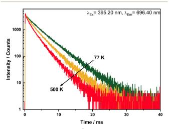
Fig. 7 Decay curves of  $LuPO_4$ :  $Eu^{3+}$ (15 mol%) sample upon excitation at 395.20 nm and emission at 696.40 nm in a temperature range between 77–500 K.
