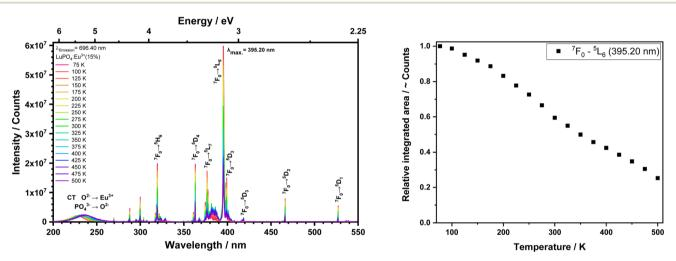
Fig. 5 Excitation spectra (left) and PL integrals (right) from the LuPO<sub>4</sub>:Eu<sup>3+</sup>(15 mol%) sample at a fixed emission wavelength at 696.40 nm in a temperature between 77 and 500 K.
