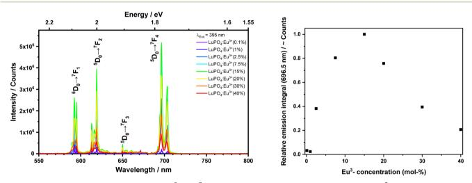
Fig. 3 Emission spectra (left) and emission integrals  $^5D_0 \rightarrow ^7F_4$  (right) upon excitation at 395 nm from the LuPO<sub>4</sub>:Eu<sup>3+</sup>(0.1–40 mol%) sample at room temperature.
