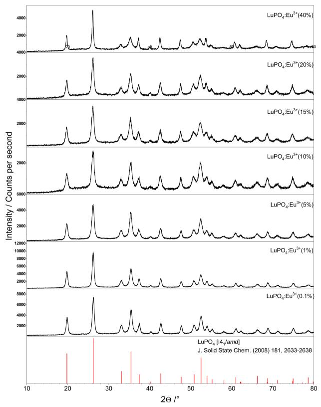
Fig. 1 Powder X-ray diffraction patterns of  $LuPO_4$ :  $Eu^{3+}$  (0.1–40 mol%) compared to the reference database pattern of tetragonal  $LuPO_4$  (mineral type: xenotime).
