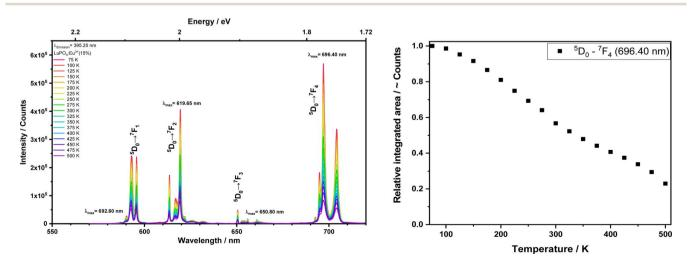
Fig. 6 Emission spectra (left) and integrals (right) from the LuPO<sub>4</sub>:Eu<sup>3+</sup>(15 mol%) sample upon excitation at 395.20 nm ( $^5$ D<sub>0</sub>  $\rightarrow$   $^7$ F<sub>4</sub>)in the temperature range between 77 and 500 K.
