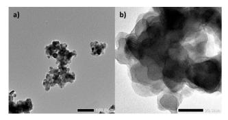
Fig. 2 TEM images of LuPO<sub>4</sub>:Eu<sup>3+</sup>(15 mol%) nanoparticles which forms agglomerates in a diameter of around 100 nm (a) while the crystallite size is about 20 nm (b).
