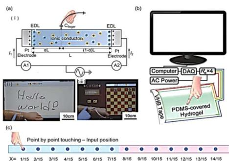
**Fig. 6** (a) The touch strip architecture (i) motion detection capabilities of the epidermal touch panel; (ii) word writing demonstrations; (iii) chess playing<sup>109</sup> (Copyright (2016) *Science*). (b) Schematic illustration showed that a wearable touch pad gets integrated into a desktop computer; (c) corresponding  $V_1$  voltage after touching each spot on the hydrogel strip with your finger<sup>110</sup> (Copyright (2020) *Advanced Materials*).
