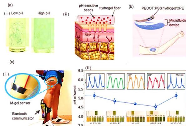
**Fig. 8** (a) (i) pH responsive bead-laden hydrogel microfibers, (ii) pH sensing hydrogel microfibers for epidermal monitoring; (b) schematic view of wearable uric acid sensor; (c) (i) wireless hydrogel sensor used for detection of muscle fatigue via pH detection, (ii) resistance changes measured over different number of movements<sup>5</sup> (Copyright (2023) *Advance materials*).
