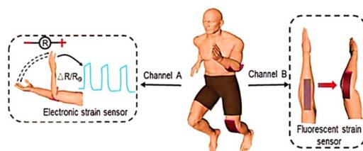
**Fig. 11** Schematic demonstration of two-way electronic and fluorescent colour reactions to motion in humans<sup>5</sup> (Copyright (2023) *Advance materials*).
