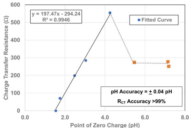
Fig. 12 A plot of each powder population's point of zero charge<sup>16</sup> against its  $R_{CT}/CPE$ . The fitted curve extends from  $pH_{PZC}$  values 1.54 to 4.25.
