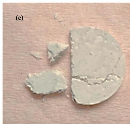
Fig. 8 (a) The Nyquist plot for the full frequency range of the run for the magnetically separated powder pellet at 0.0 V bias. (b) The high frequency range for the Nyquist plot shows only  $R_s$ ,  $Z_L$ , and  $Z_w$ . The signal distortion was caused by the pellet fracturing during this second run at 0.0 V bias. (c) The magnetically separated pellet that fractured during the run at 0.0 V bias, causing the signal distortion.
