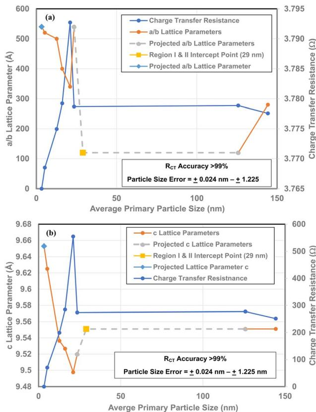
Fig. 14 (a) Direct comparison of the  $R_{CT}/CPE$  and  $a/b$  lattice parameters<sup>16</sup> for all the sample populations measured. (b) A direct comparison of the  $R_{CT}/CPE$  and the  $c$  lattice parameters<sup>16</sup> for all the samples measured.
