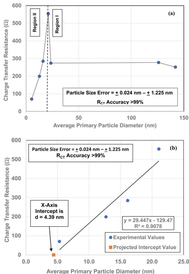
Fig. 4 (a) A plot of all the powder population's charge transfer resistance ( $R_{CT}/CPE$ ) values against their average primary particle diameter for Regions I and II. (b) The  $R_{CT}/CPE$  values for the linear portion of the curve (below  $d = 21.08$  nm) in Region II. The plot was used to obtain a projected average particle diameter where  $R_{CT}/CPE$  might go to zero.
