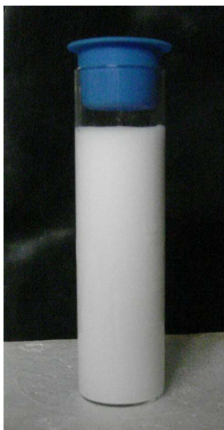
Fig. 19 Disbursed anatase titania in deionized water for particle settling while not in the presence of a magnetic field.
