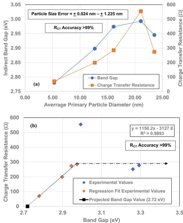
Fig. 13 (a) Bandgap<sup>16</sup> and  $R_{CT}/CPE$  values plotted against their average primary particle diameter. (b) Bandgap values<sup>16</sup> plotted against their  $R_{CT}/CPE$ . The projected band gap value of 2.72 eV is for  $R_{CT}/CPE = 0.0$   $\Omega$ .
