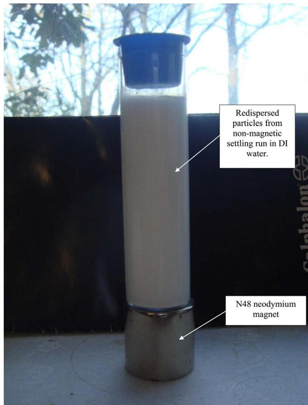
Fig. 23 Redispersed particles from non-magnetic settling run.
