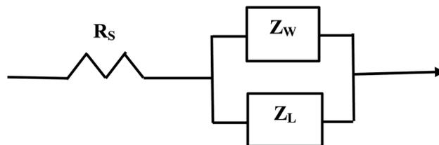
Fig. 10 The equivalent circuit of the curves in Fig. 7(a)–(c) through Fig. 9(a) and (b). Solution resistance ( $R_s$ ) is measured from the origin to where the highest frequency point is recorded intercepting the real axis ( $Z'$ ). Beyond  $R_s$  on the  $Z'$  axis are the summed values of  $Z_L$  and  $Z_w$  across the same frequency range.
