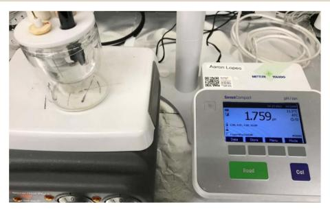
Fig. 1 The electrical cell, clamped pellet, and pH/ion meter set-up for the EIS system used to obtain a Nyquist plot.
