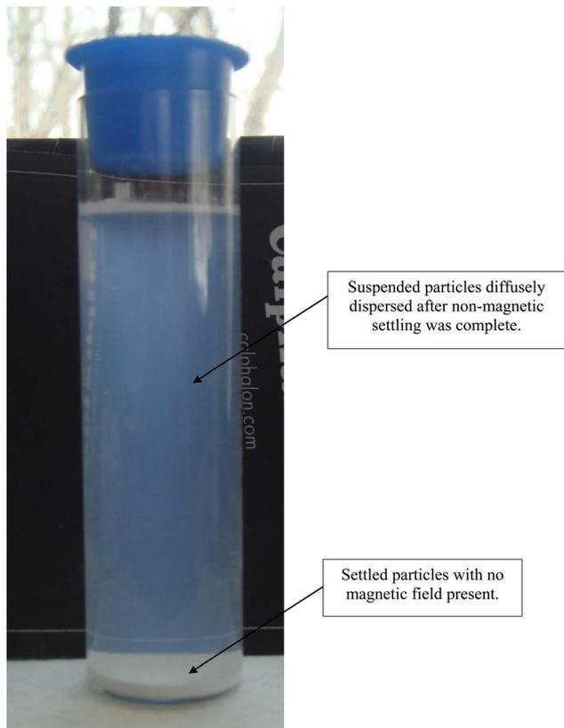
Fig. 20 Anatase titania in deionized water while not in a magnetic field during settling while exposed to ambient light at 36 days.
