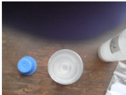
Fig. 17 A view of the powder circles created by settling particles before the solution was removed on day 43. The concentric rings demonstrate how the settled particles were rejected by the strongest portion of the magnetic field during settling.
