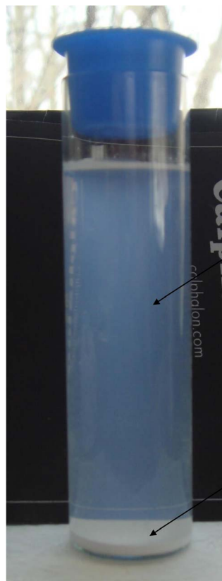
Fig. 20 Anatase titania in deionized water while not in a magnetic field during settling while exposed to ambient light at 36 days.
