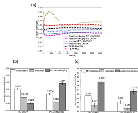
**Fig. 5** Friction and wear of different treated PE-UHMW and PE-UHMW/GO composites under lubrication with water: (a) friction coefficient vs. time curve, (b) average friction coefficient, (c) average wear rate.
