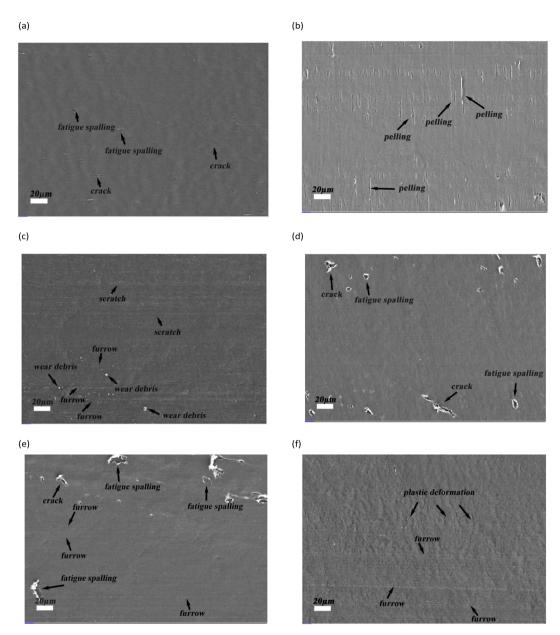
Fig. 6 SEM images (1000× magnification) of the worn surface of different treated PE-UHMW and PE-UHMW/GO composites under water lubrication: (a) PE-UHMW, (b) PE-UHMW/GO, (c) irradiated PE-UHMW, (d) irradiated PE-UHMW/GO, (e) aged PE-UHMW, (f) aged PE-UHMW/GO, (e) aged PE-UHMW/GO, (e) aged PE-UHMW/GO, (f) aged PE-UHMW/GO, (g) GO.
