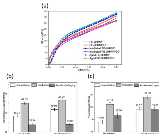
Fig. 4 Impressive properties of different treated PE-UHMW/GO and PE-UHMW composites: (a) compressive stress–strain curve, (b) compressive strength, (c) yield strength.
