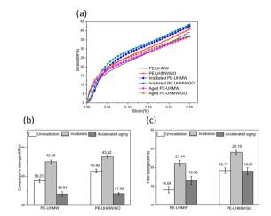
Fig. 4 Impressive properties of different treated PE-UHMW and PE-UHMW/GO composites: (a) compressive stress-strain curve, (b) compressive strength, (c) yield strength.
