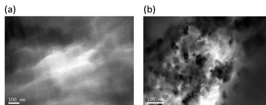
Fig. 3 TEM images: (a) PE-UHMW, (b) PE-UHMW/GO composites.
