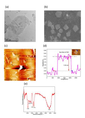
**Fig. 2** Morphological characterization of GO: (a) TEM image of GO, (b) SEM image of GO, (c) AFM image of GO, (d) the thick of GO, (e) FTIR spectroscopy of GO.
