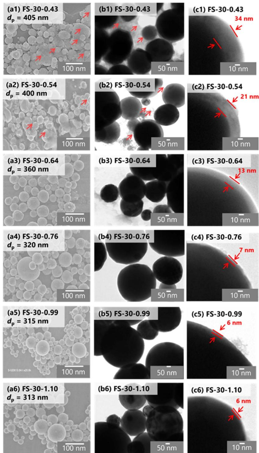
Fig. 5 The effect of the number of cores on the morphology of Fe@SiO<sub>2</sub> particles. (a) SEM and TEM images of Fe@SiO<sub>2</sub> particles at a different number of cores: (1)  $0.43 \times 10^6$ , (2)  $0.54 \times 10^6$ , (3)  $0.64 \times 10^6$ , (4)  $0.76 \times 10^6$ , (5)  $0.99 \times 10^6$  and (6)  $1.10 \times 10^6$  cores per cm<sup>3</sup> carrier gas at (b) low magnification and (c) high magnification.
