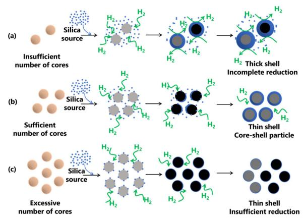
Fig. 8 Proposed mechanism for the formation of SiO<sub>2</sub>-coated Fe with (a) insufficient, (b) sufficient, and (c) excessive number of cores.
