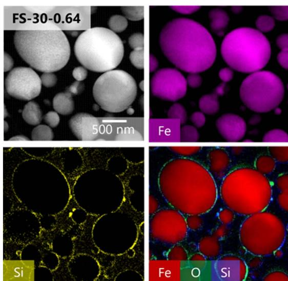
Fig. 6 TEM image and elemental mapping of the cross-section of Fe@SiO<sub>2</sub> particles (FS-30-0.64).
