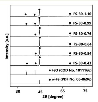
Fig. 4  $\,$  XRD patterns of samples prepared using 30% (v/v) of ethanol with different number of cores.
