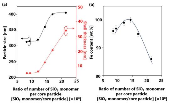
Fig. 7 Correlation between the number of  $SiO_2$  monomer per core particle ratios on the (a) particle size and shell thickness and (b)  $\alpha$ -Fe content in the Fe@SiO $_2$  particles.
