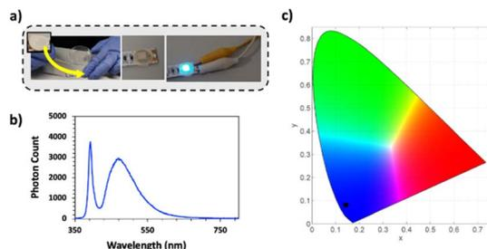
Fig. 7 (a) Representative image of the integration of the color-converting *P. harmala* embedded paper with the LED, (b) LED emission spectrum under 5 mA current flow, and (c) CIE 1931 color coordinates of the obtained LED on the chromaticity diagram.
