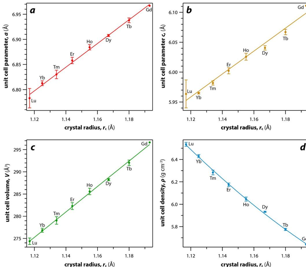
Fig. 5 Relationships of (a and b) unit cell parameters, (c) unit cell volumes, and (d) densities with respect to RE  $r_c$  of xenotime compounds. Where multiple values were given, averages and standard deviations are reported.
