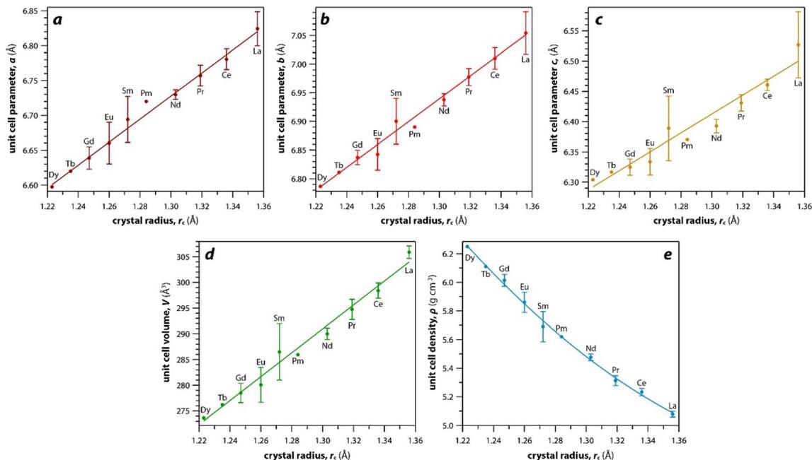
Fig. 3 Relationships of (a–c) unit cell parameters, (d) unit cell volumes, and (e) densities with respect to RE  $r_c$  of monazite compounds. Where multiple values were given, averages and standard deviations are reported.
