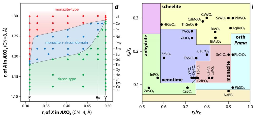
**Fig. 6** (a) Structure-field map of monazite and xenotime compounds based on the ionic radius ( $r_i$ ) of A (e.g., RE) and X (e.g., P) in  $\text{AXO}_4$  compounds.<sup>107</sup> Reprinted with permission from Aldred.<sup>107</sup> Copyright 1984 American Chemical Society. (b) Modified Bastide diagram for  $\text{ABX}_4$  compounds. Reprinted with permission from Hay *et al.*<sup>115</sup> Copyright 2013 Elsevier.
