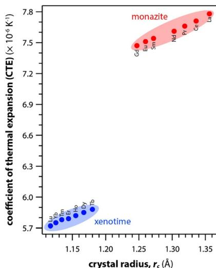
**Fig. 8** Summary of calculated CTE values for both monazite and xenotime REPO<sub>4</sub> crystals from Li *et al.*<sup>121</sup> as a function of RE  $r_c$ .
