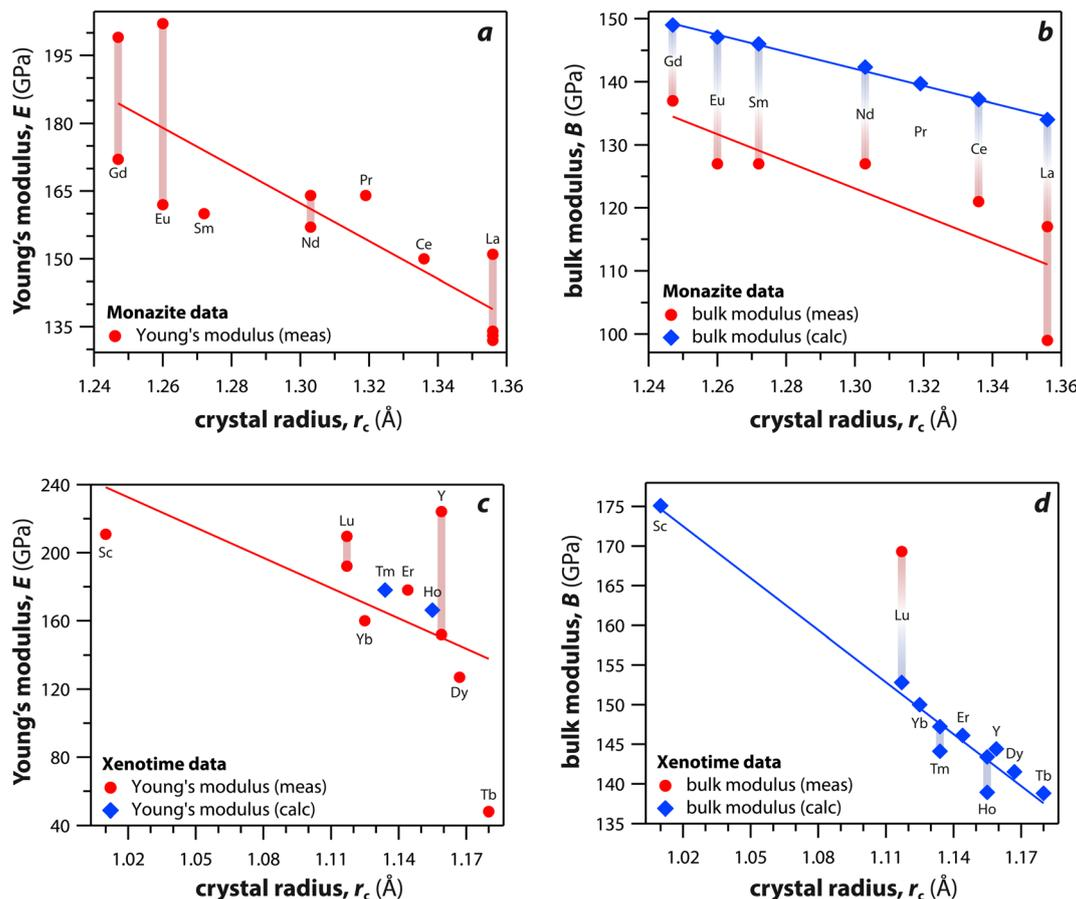
Fig. 7 (a and c) Young's modulus and (b and d) bulk modulus values of (a and b) monazite and (c and d) xenotime compounds as functions of crystal radius of the RE cation ( $r_c$ ).
