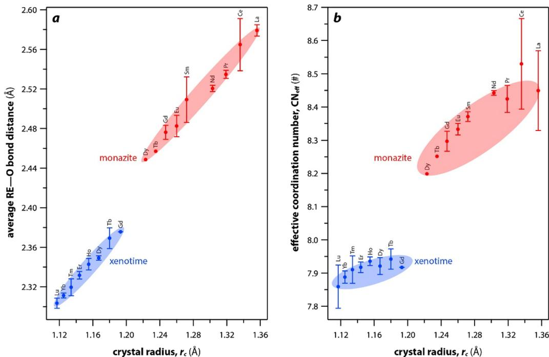
Fig. 4 (a) Average RE–O bond distances and (b) effective coordination numbers of REO<sub>x</sub> polyhedral with respect to RE  $r_c$  in monazite and xenotime structures.
