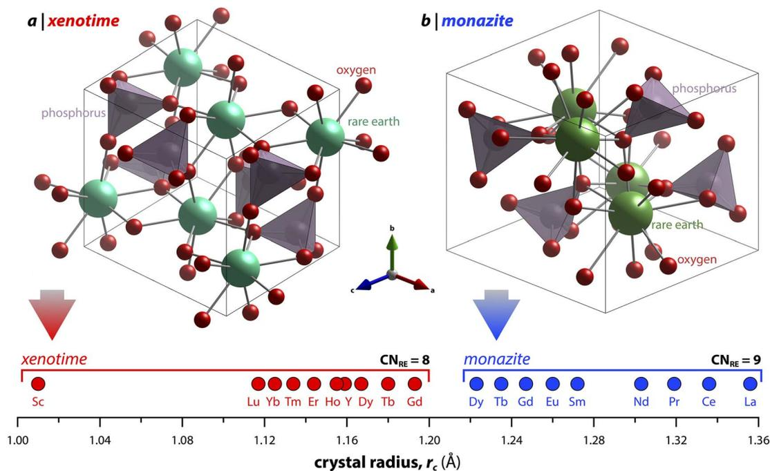
Fig. 1 Illustration showing the relationship of (a) xenotime and (b) monazite structures of REPO<sub>4</sub> to the RE crystal radii ( $r_c$ ) from Shannon.<sup>49</sup> LuPO<sub>4</sub> (ICSD 46792) and LaPO<sub>4</sub> (ICSD 46788) were used to create the (a) xenotime and (b) monazite unit cell structures, respectively.
