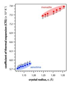
Fig. 8 Summary of calculated CTE values for both monazite and xenotime REPO<sub>4</sub> crystals from Li et al.  $^{121}$  as a function of RE  $r_{\rm c}$ .
