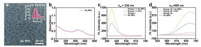
Fig. 4 Inner filter effect. (a) HRTEM images and particle size (inset) of Au NPs. (b) UV-vis absorption spectrum of Au NPs. (c) Photoemission spectra of Group 1 after adding Au NPs ( $\lambda_{ex} = 338$  nm). (d) Photoemission spectra of Group 10 after adding Au NPs ( $\lambda_{ex} = 500$  nm). All photoemission spectra were slit widths of excitation: 5 nm, slit widths of emission: 5 nm, and voltage: 600 V.
