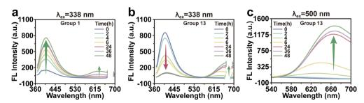
Fig. 5 Growth mechanism of BSA-Au NCs. (a) Photoemission spectra of Group 1 with time-dependent ( $\lambda_{ex} = 338$  nm). (b and c) Photoemission spectra of Group 13 with time-dependent ( $\lambda_{ex} = 338$  nm and 500 nm). All photoemission spectra were slit widths of excitation: 5 nm, slit widths of emission: 5 nm, and voltage: 600 V.
