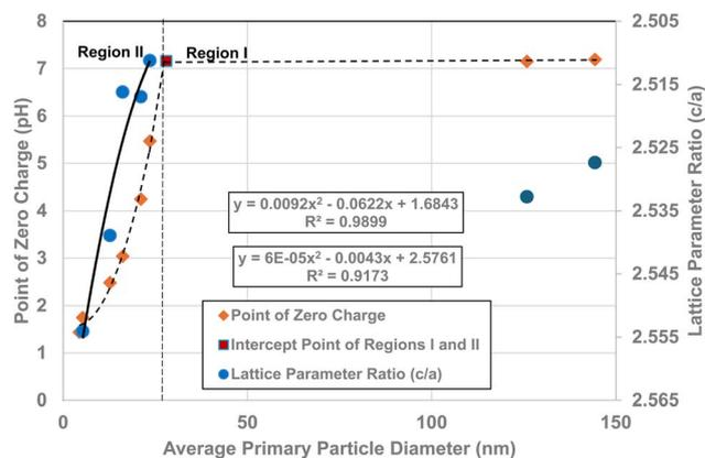
Fig. 6 A visual correlation between the experimental lattice parameter ratios ( $c/a$ ) and experimental PZC values against their average primary particle diameters. The lattice parameter ratios ( $c/a$ ) values are reversed to provide a clearer visual correlation with their PZC values.
