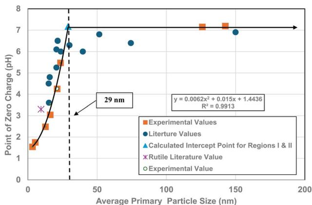
Fig. 4 Values for both experimental and literature<sup>124–134</sup>  $\text{pH}_{\text{PZC}}$  values are plotted against their normalized average primary particle diameter. The experimental point at  $\text{pH}_{\text{PZC}} = 4.26$  was measured using 0.1 M NaOH for the electrolyte, and 0.01 M  $\text{NaClO}_4$  as the titrant.<sup>134</sup>
