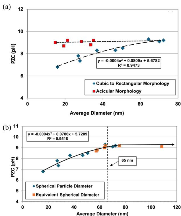
Fig. 1 (a) Correlation between the calculated average primary particle spherical diameters using specific surface area plotted against their PZC values for Groups 1 & 2 of synthetic goethite ( $\alpha\text{-FeO(OH)}$ ).<sup>47–59</sup> (b) Correlation between the spherical to rectangular particle diameters with the normalized acicular particle diameters against their PZC values for Groups 1 & 2 of goethite ( $\alpha\text{-FeO(OH)}$ ).<sup>47–59</sup>
