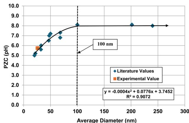
Fig. 11 A plot of the average primary particle size against their PZC values for monoclinic zirconia ( $\text{ZrO}_2$ ).<sup>73–85</sup> The method presented in Section A.1 was used to obtain the average diameter of each data set. The experimental point was measured in 0.1 M  $\text{NaClO}_4$  electrolyte using 0.01 M NaOH as the titrant.<sup>134</sup>
