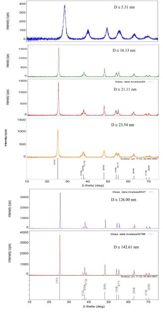
Fig. 21 PXRD patterns for each of the samples used in this work, save Fig. 2. Each pattern fits the PXRD pattern JCPDS #00-064-0863 for synthesized anatase titania.  $^{120}$
