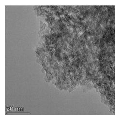
Fig. 13 Powder population 1 with an average primary particle diameter of 5.307 nm  $\pm$  0.527 nm.
