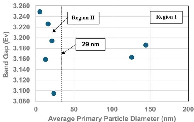
Fig. 28 Indirect band gap values of anatase titania prepared by pressing each sample at 10 tons.<sup>119</sup>
