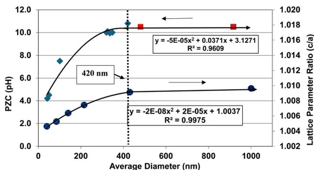
Fig. 8 Plots of the average primary particle size, PZC values and their lattice parameter ratio ( $c/a$ ) for  $\text{BaTiO}_3$ .<sup>61–72</sup> The method presented in Section A.1 was used to obtain the average diameter of each data set. The two sets of data were plotted together so a visual correlation could be obtained.
