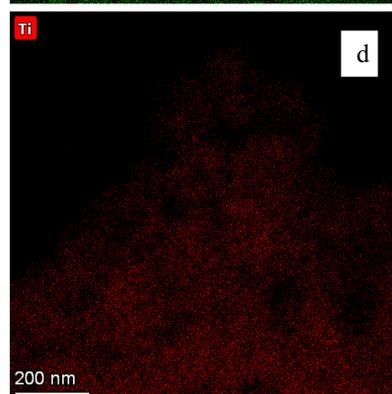
Fig. 20 (a–d) Are the EDS micrographs of the powder population in Fig. 13. (b) The EDS micrographs for  $\text{Ti}^{4+}$  and  $\text{O}^{2-}$ . (c) The EDS micrograph for  $\text{O}^{2-}$  and (d) the EDS micrograph for  $\text{Ti}^{4+}$  (d). No trace elements were found in figures (b)–(d).
