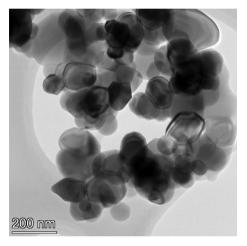
Fig. 19 Powder population 7 with an average primary particle diameter of 142.614 nm  $\pm$  37.092 nm.
