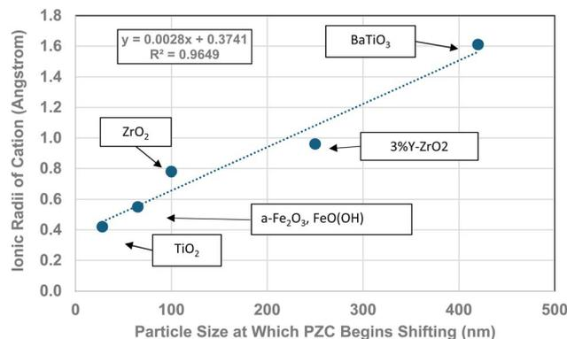
Fig. 12 The effect of the largest cation ionic radius on the particle size at which the metal-oxide PZC values begin to decrease.<sup>110</sup>
