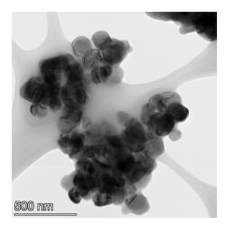
Fig. 18 Powder population 6 with an average primary particle diameter of 126.002 nm  $\pm$  29.775 nm.
