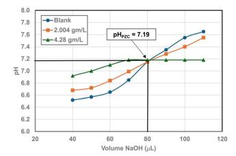
Fig. 27 Mass titration curves of anatase titania with an average primary particle with a  $d\cong 142.614$  nm. Intersection of the three curves indicate the materials pH<sub>PZC</sub> = 7.19.
