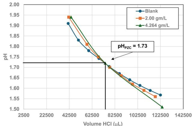
Fig. 22 Mass titration curves of anatase titania with an average primary particle with a  $d \approx 5.307$  nm. Intersection of the three curves indicate the materials  $\text{pH}_{\text{PZC}} = 1.73$ . The large volume of HCl (0.01 N) titrant used was due to its low molar concentration.
