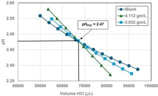
Fig. 3 Mass titration curves of anatase titania with an average primary particle with a  $d \cong 12.69$  nm. Intersection of the three curves indicate the materials  $pH_{PZC} = 2.47$ .
