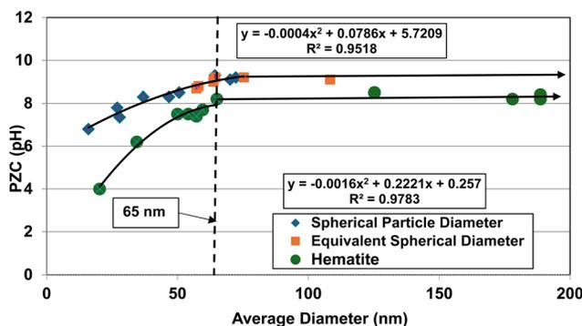
Fig. 9 Plots of the average primary particle size against their PZC values for goethite (upper curve)<sup>47–59</sup> and hematite (lower curve)<sup>86–95</sup> were plotted together so the results could be visually correlated. The method presented in Section A.1 was used to obtain the average diameter of each data set.
