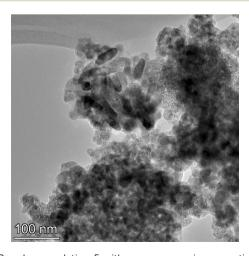
Fig. 17 Powder population 5 with an average primary particle diameter of 23.538 nm  $\pm$  4.044 nm.
