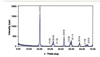
Fig. 2 The PXRD pattern for the sample with an average diameter ≈12.69 nm. The indexed peaks fit those in the JCPDS file #00-0634-0863 (ref. 120) for synthetic anatase titania.
