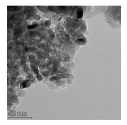
Fig. 14 Powder population 2 with an average primary particle diameter of 12.689 nm  $\pm$  2.400 nm.
