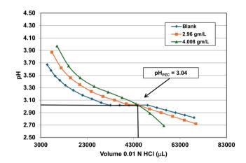
Fig. 23 Mass titration curves of anatase titania with an average primary particle with a  $d \cong 16.131$  nm. Intersection of the three curves indicate the materials pH<sub>PZC</sub> = 3.04. The large volume of HCl (0.01 N) titrant used was due to its low molar concentration.
