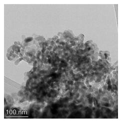
Fig. 16 Powder population 4 with an average primary particle diameter of 21.108 nm  $\pm$  4.059 nm.
