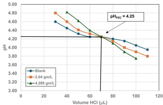
Fig. 24 Mass titration curves of anatase titania with an average primary particle with a  $d \approx 21.108$  nm. Intersection of the three curves indicate the materials  $\text{pH}_{\text{PZC}} = 4.25$ .
