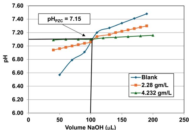
Fig. 26 Mass titration curves of anatase titania with an average primary particle with a  $d \approx 126.002$  nm. Intersection of the three curves indicate the materials  $\text{pH}_{\text{PZC}} = 7.15$ .
