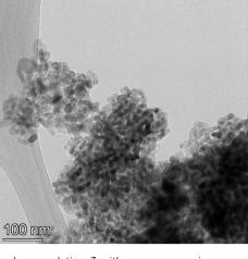
Fig. 15 Powder population 3 with an average primary particle diameter of 16.131 nm  $\pm$  3.958 nm.
