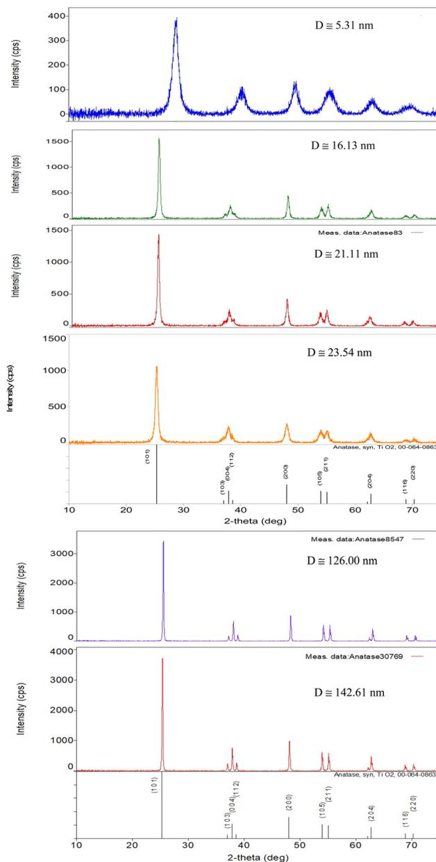
**Fig. 21** PXRD patterns for each of the samples used in this work, save Fig. 2. Each pattern fits the PXRD pattern JCPDS #00-064-0863 for synthesized anatase titania.<sup>120</sup>
