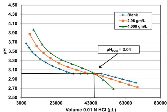
Fig. 23 Mass titration curves of anatase titania with an average primary particle with a  $d \approx 16.131$  nm. Intersection of the three curves indicate the materials  $\text{pH}_{\text{PZC}} = 3.04$ . The large volume of HCl (0.01 N) titrant used was due to its low molar concentration.
