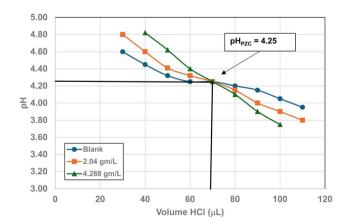
Fig. 24 Mass titration curves of anatase titania with an average primary particle with a  $d \cong 21.108$  nm. Intersection of the three curves indicate the materials  $pH_{PZC} = 4.25$ .
