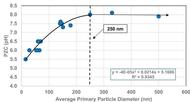
Fig. 10 A plot of the average primary particle size and PZC values for 3% doped tetragonal  $\text{ZrO}_2$ .<sup>96–109</sup> The method presented in Section A.1 was used to obtain the average diameter of each data set.
