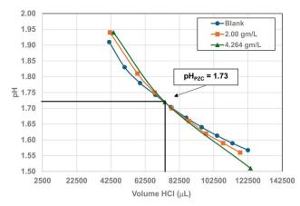
Fig. 22 Mass titration curves of anatase titania with an average primary particle with a  $d \cong 5.307$  nm. Intersection of the three curves indicate the materials pH<sub>PZC</sub> = 1.73. The large volume of HCl (0.01 N) titrant used was due to its low molar concentration.
