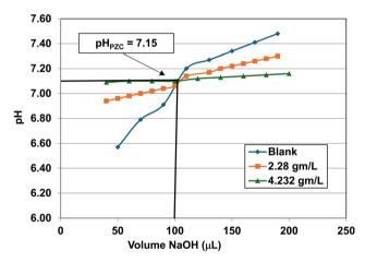
Fig. 26 Mass titration curves of anatase titania with an average primary particle with a  $d \cong 126.002$  nm. Intersection of the three curves indicate the materials pH<sub>PZC</sub> = 7.15.
