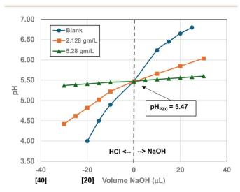
Fig. 25 Mass titration curves of anatase titania with an average primary particle of  $d\cong 23.538$  nm. Intersection of the three curves indicates the materials  $pH_{PZC}=5.46$ .
