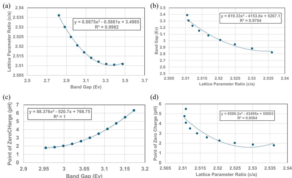
Fig. 7 (a) Plot of the calculated band gap values against the lattice parameter ratio ( $c/a$ ) in Region II. (b) Plot of the calculated lattice parameter ratio ( $c/a$ ) against its band gap (eV) in Region II. (c) Quantitative correlation between the calculated surface band gap (*i.e.*, bond lengths) and their PZC values in Region II. (d) Quantitative correlation between calculated lattice parameter ratio ( $c/a$ ) and point of zero charge values in Region II.
