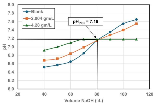
Fig. 27 Mass titration curves of anatase titania with an average primary particle with a  $d \approx 142.614$  nm. Intersection of the three curves indicate the materials  $\text{pH}_{\text{PZC}} = 7.19$ .
