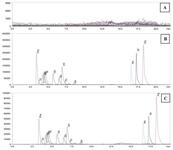
Fig. 1 Simple mass chromatogram of 13 amino acids of (A) blank, (B) spike-100 μM concentration and (C) STD-100 μM concentration using LCMS/MS system.
