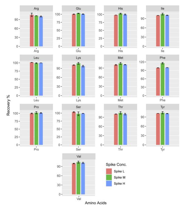
Fig. 4 Recovery for the analysis of each amino acid (n = 3).
