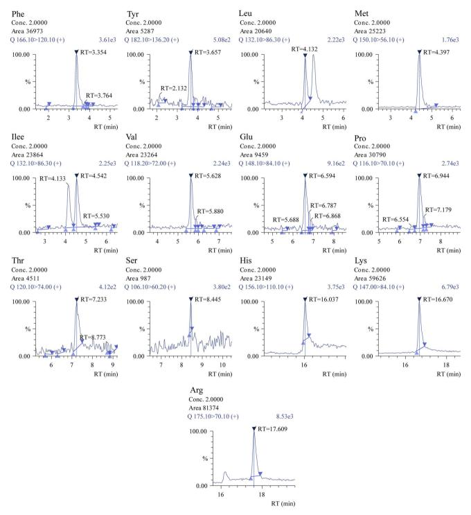
Fig. 6 Chromatograms of compounds of interest obtained using the Shimadzu insight software. Analysis was performed using 2  $\mu$ M concentration (other amino acids in ESI 02†) for the comparative study of targeted amino acids.
