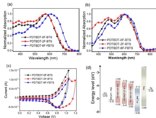
Fig. 1 Absorption spectra of the copolymer in solution (a) and in solid film (b). Cyclic voltammogram (c) and energy level schematic (d) of material in this work.
