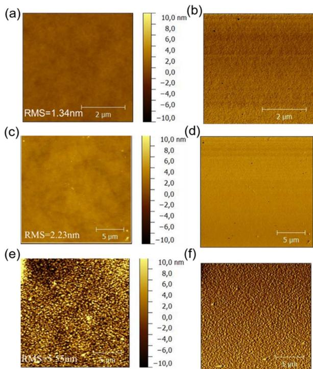
Fig. 9 AFM height images and phase images of the PDTBDT-0F-BTS:PC<sub>71</sub>BM (a) and (b), PDTBDT-2F-BTS:PC<sub>71</sub>BM (c) and (d) and PDTBDT-6F-FBTS:PC<sub>71</sub>BM (e) and (f).
