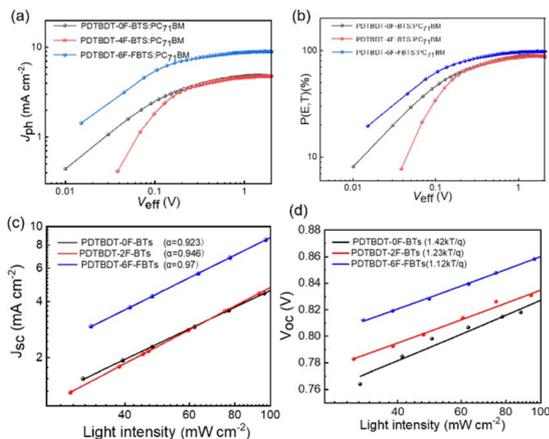
Fig. 7 The curves of  $J_{ph}$ – $V_{eff}$  (a);  $P(E, T)$ – $V_{eff}$  plots (b);  $V_{oc}$  (c) and  $J_{sc}$  (d) versus the natural logarithm of light intensities of optimised devices characteristics of the inverted PVCs from the three copolymers with 2% DIO additive under AM 1.5G illumination ( $100 \text{ mW cm}^{-2}$ ).
