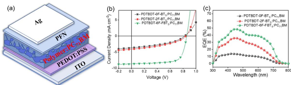
Fig. 6 Device structure diagram (a); the optimized current density–voltage ( $J$ - $V$ ) curves (b); the EQE spectra (c).
