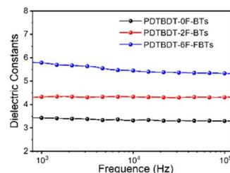
Fig. 2 Variation of the relative dielectric constants of the copolymers with frequency.
