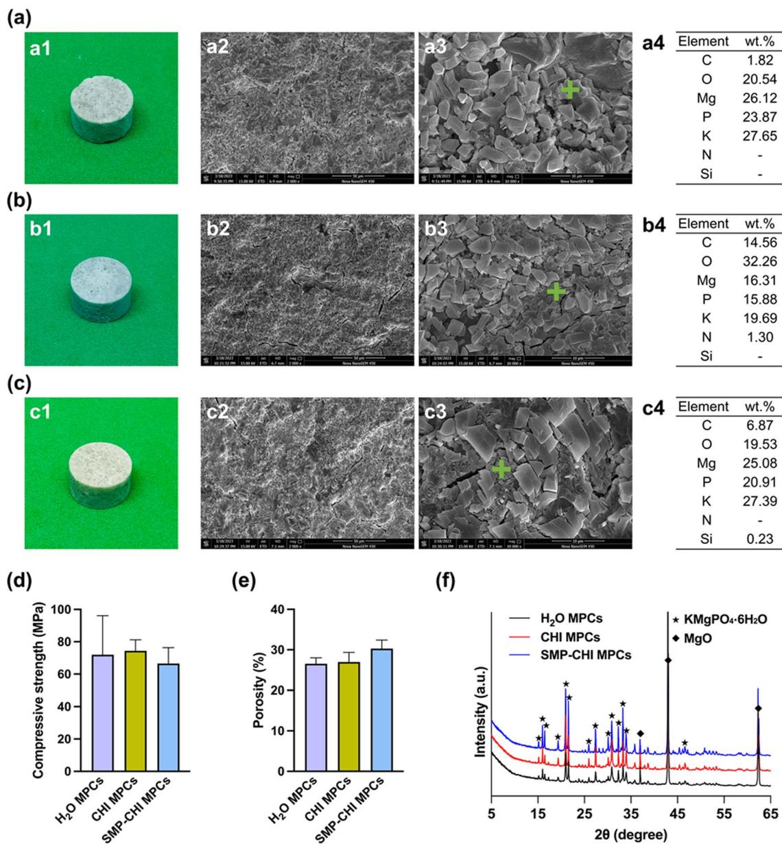
Fig. 3 Optical images, morphologies, and EDS analyses of (a) H<sub>2</sub>O MPC, (b) CHI MPC, and (c) SMP-CHI MPC. (d) Compressive strength of the cements. (e) Porosity of MPCs. (f) XRD of different samples.
