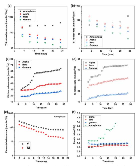
Fig. 8 Leached samples short-term (1 day) release rate of (a) Y and (b) Si.  $\alpha$ ,  $\beta$ , and  $\gamma$ -phase  $Y_2Si_2O_7$  long-term (28 days) release rates of (c) Y and (d) Si. (e) Amorphous  $Y_2Si_2O_7$  long-term (20 days) release rates of Y and Si; and (f) long-term atomic ratio (Y/Si) of amorphous,  $\alpha$ ,  $\beta$  and  $\gamma$ -phase  $Y_2Si_2O_7$  samples.
