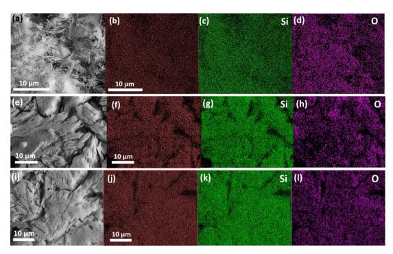
Fig. 4 SEM images and EDS mappings of the  $\alpha$ ,  $\beta$ , and  $\gamma$ -phase  $Y_2Si_2O_7$  pellets after the 28 days leaching tests at 90 °C in a solution of nitric acid at pH = 3.0. Images (a-d), (e-h), and (i-l) correspond to the  $\alpha$ ,  $\beta$  and  $\gamma$ -phase respectively.
