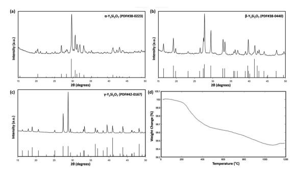
Fig. 2 (a–c) XRD patterns of sintered α, β, and  $\gamma$ -phase  $Y_2Si_2O_7$  pellets, (d) thermogravimetric analysis of  $Y_2Si_2O_7$  powders from room temperature to 1200 °C.
