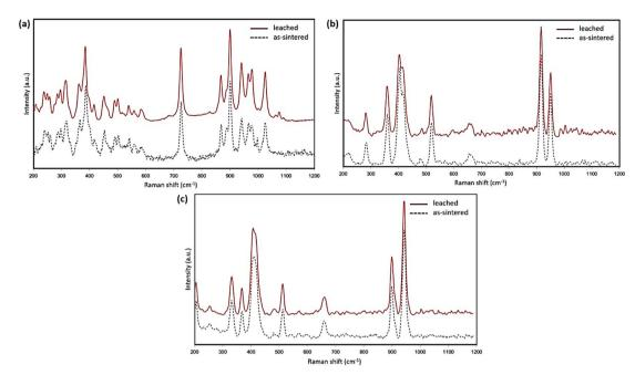
Fig. 5 Raman spectra of the  $\alpha$  (a),  $\beta$  (b), and  $\gamma$  (c) phase  $Y_2Si_2O_7$  pellets before and post-leaching tests in pH = 3.0 nitric acid for 28 days at 90 °C.
