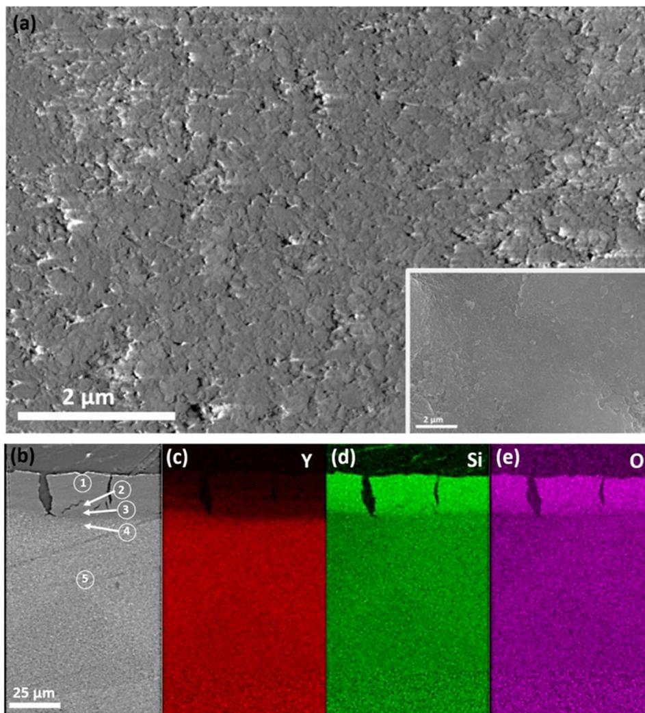
Fig. 7 (a) SEM images showing the pristine sintered amorphous  $\text{Y}_2\text{Si}_2\text{O}_7$  pellet and the pellets after the 20 days leaching tests at 90 °C in a solution of nitric acid at pH = 3.0 respectively. (b) A SEM image of the amorphous pellet in a cross-sectional view and the corresponding EDS mappings of the cross-section (c–e).
