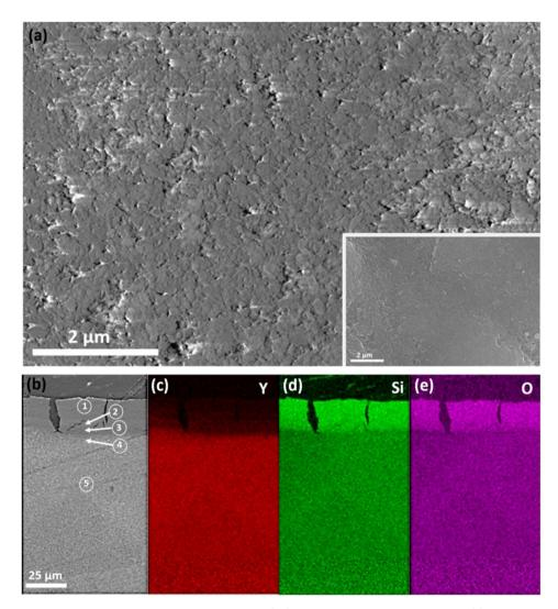
Fig. 7 (a) SEM images showing the pristine sintered amorphous  $Y_2Si_2O_7$  pellet and the pellets after the 20 days leaching tests at 90 °C in a solution of nitric acid at pH = 3.0 respectively. (b) A SEM image of the amorphous pellet in a cross-sectional view and the corresponding EDS mappings of the cross-section (c-e).
