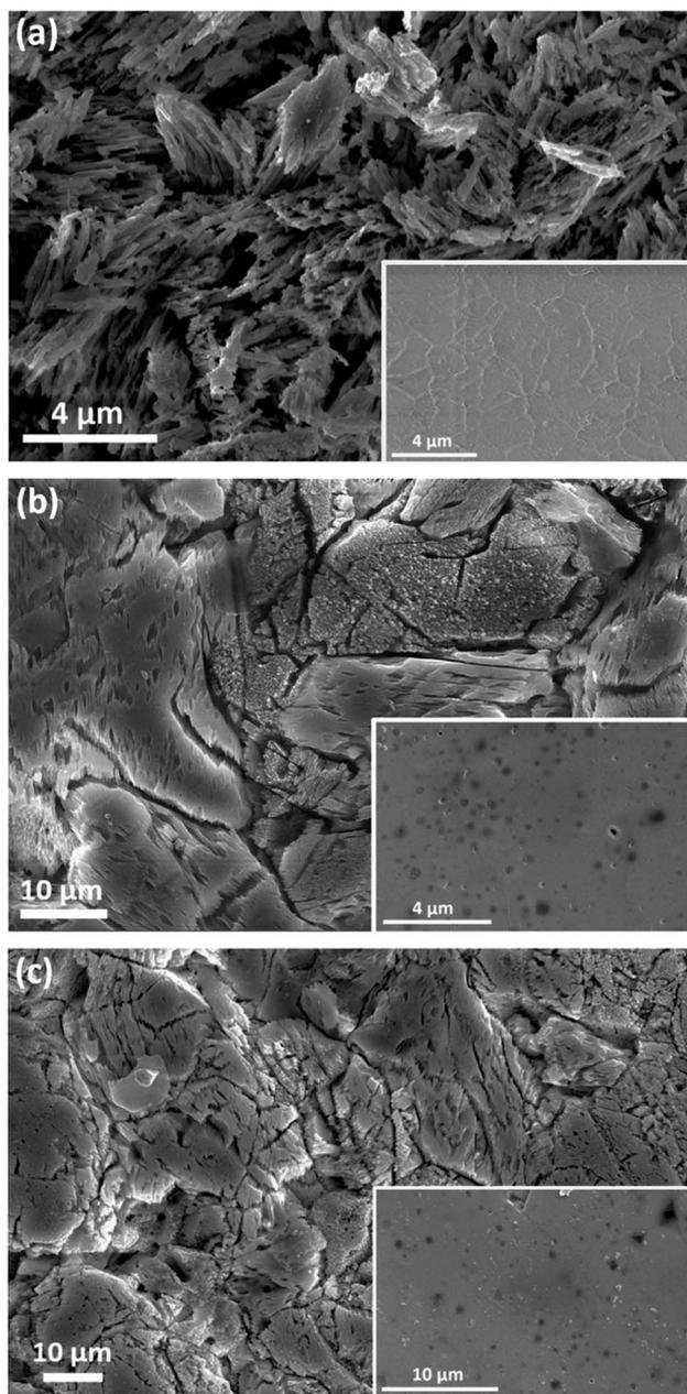
Fig. 3 (a–c) SEM images showing the surface morphological variation of the  $\alpha$ ,  $\beta$ , and  $\gamma$ -phase  $Y_2Si_2O_7$  pellets respectively. The smaller SEM images show the pristine sintered pellets, while the large images show the pellets after the 28 days leaching tests at 90 °C in a solution of nitric acid at pH = 3.0.
