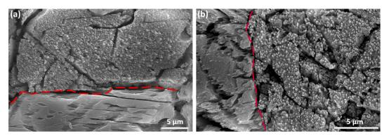
Fig. 6 (a and b) SEM images showing the post-leaching surface morphology variation of the  $\beta$  and  $\gamma$ -phase  $Y_2Si_2O_7$  pellets respectively.
