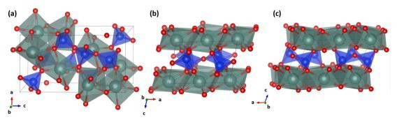
Fig. 1 Diagrams of the  $\alpha$ ,  $\beta$ , and  $\gamma$ -phase  $Y_2Si_2O_7$  structures. The green, blue, and red spheres represent Y, Si, and oxygen atoms, respectively.
