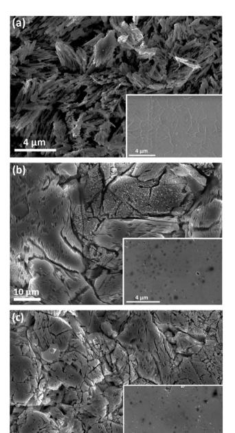
Fig. 3 (a–c) SEM images showing the surface morphological variation of the  $\alpha$ ,  $\beta$ , and  $\gamma$ -phase  $Y_2Si_2O_7$  pellets respectively. The smaller SEM images show the pristine sintered pellets, while the large images show the pellets after the 28 days leaching tests at 90 °C in a solution of nitric acid at pH =3.0.
