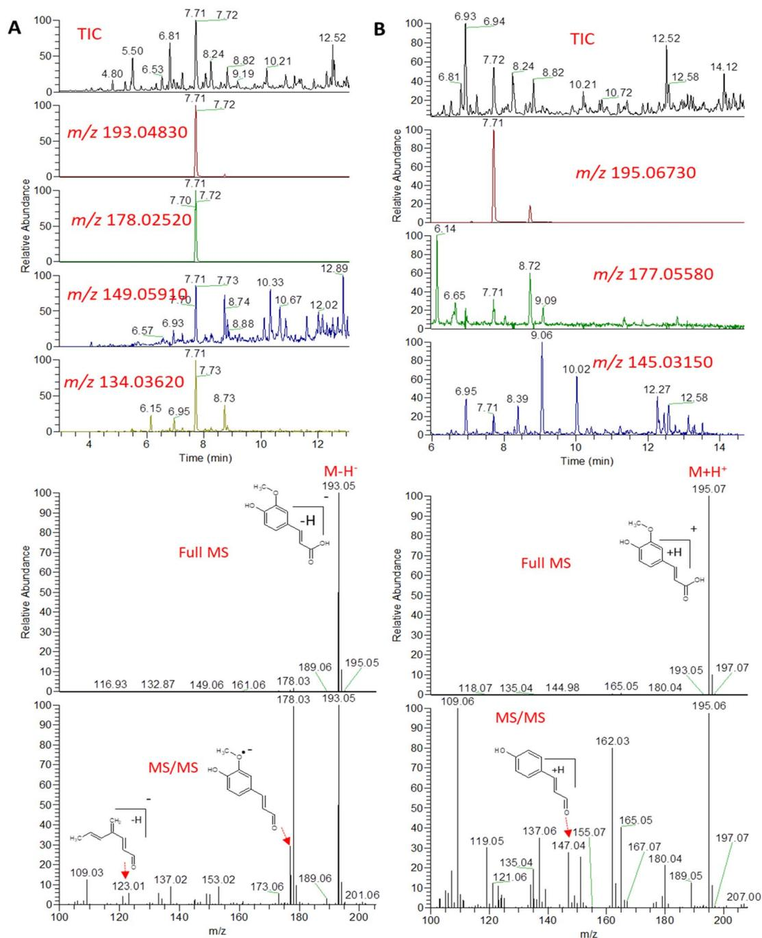
Fig. 2 Total ion chromatogram (TIC) and extracted ion chromatograms (EIC) of the peak representing ferulic acid measured by UPLC-MS-MS in negative (A) and positive (B) ionization mode from *A. nidulans* extract.
