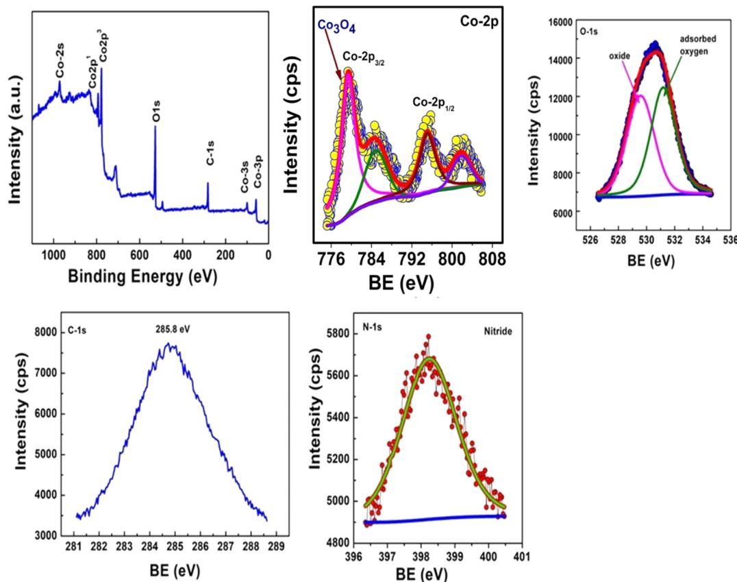
Fig. 5 XPS survey spectrum of 10CN–Co<sub>3</sub>O<sub>4</sub>, & high-resolution spectra for Co 2p, O 1s, C 1s and N 1s.
