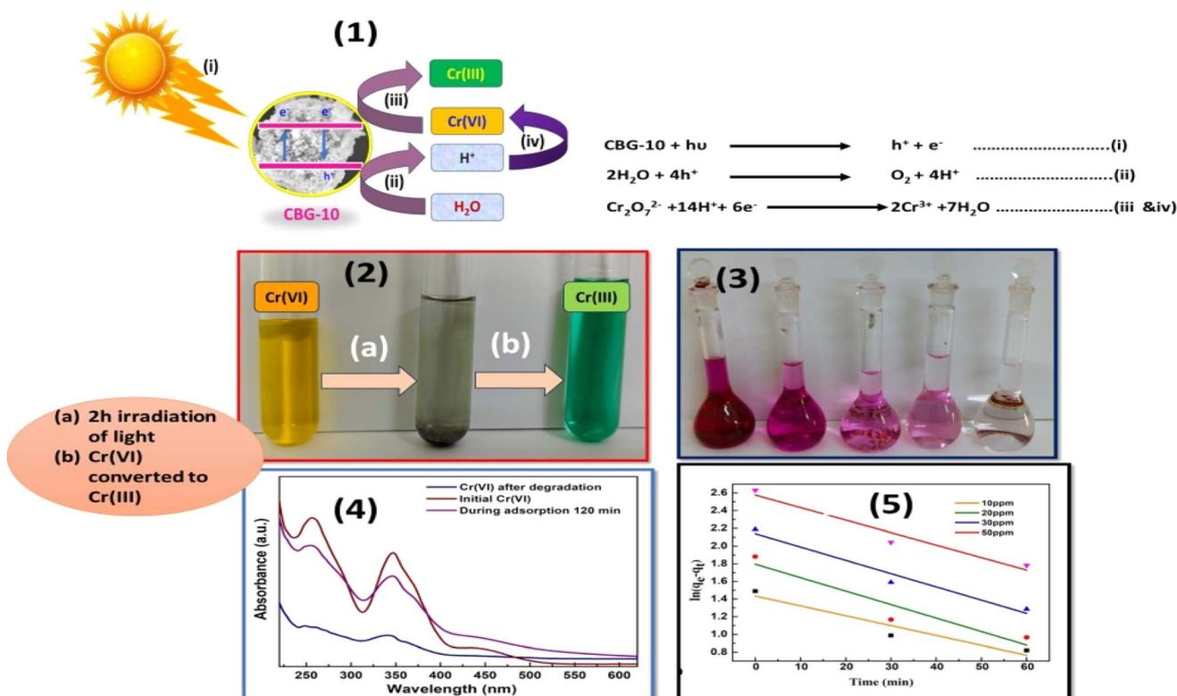
Fig. 13 (1) Schematic representation of plausible reaction mechanism of photocatalytic reduction of Cr(vi) to Cr(III) under the illumination of light by CBG-10; (2)–(4) photo reduction of Cr(vi) to Cr(III) and (5) pseudo first order linear fit with varying concentration.
