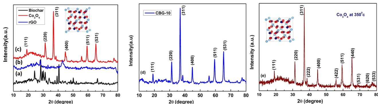
Fig. 1 XRD analysis of (a) biochar (b) rGO (c) Co<sub>3</sub>O<sub>4</sub> at 500 °C (d) CBG-10 and (e) Co<sub>3</sub>O<sub>4</sub> at 350 °C nanocomposite photocatalyst.
