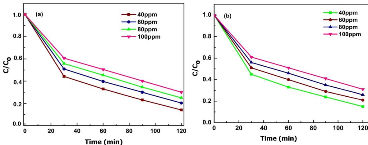
Fig. 11 Effect of illumination time of photodegradation of MG (a) and MB (b) at different initial concentrations by CBG-10.
